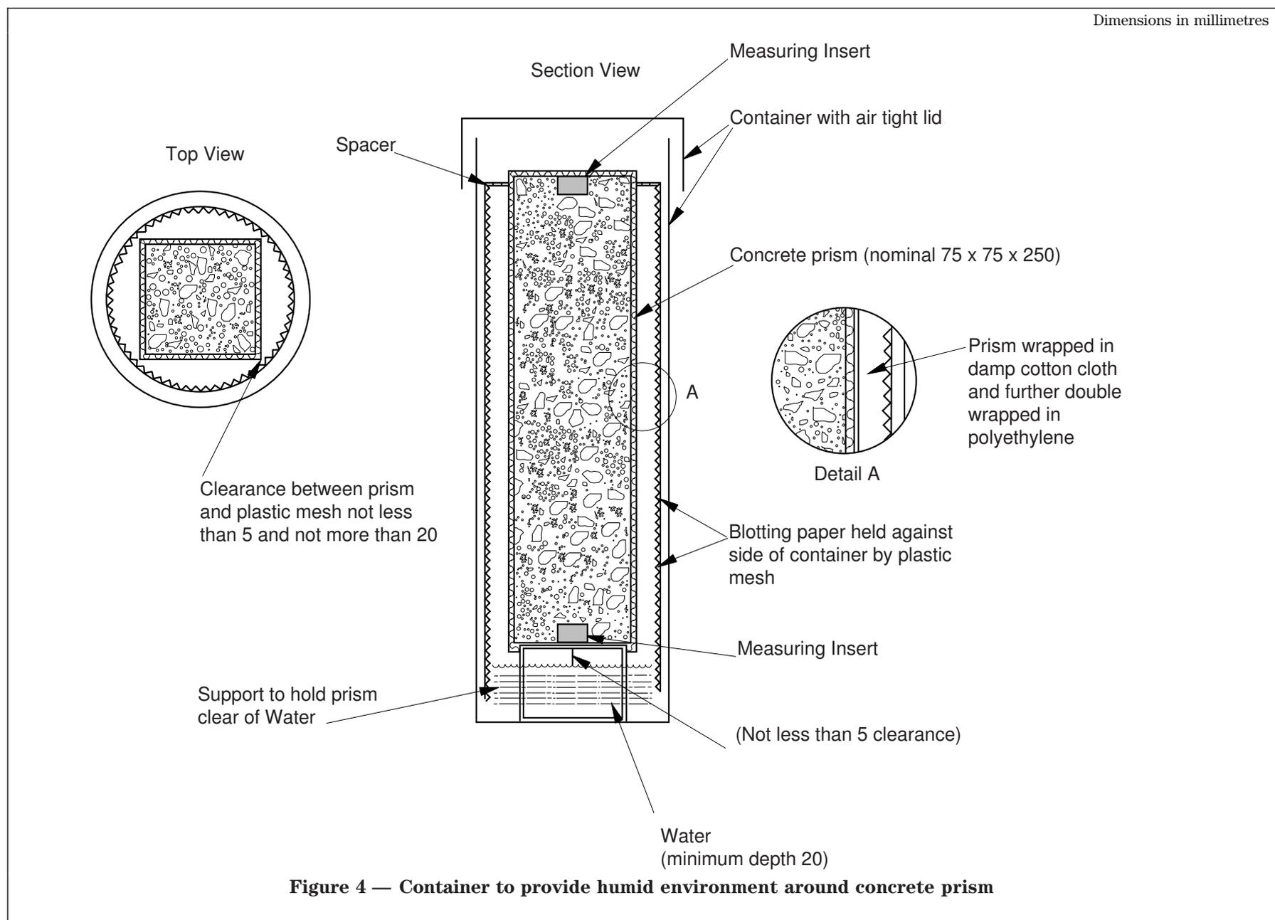
Figure 4 — Container to provide humid environment around concrete prism
