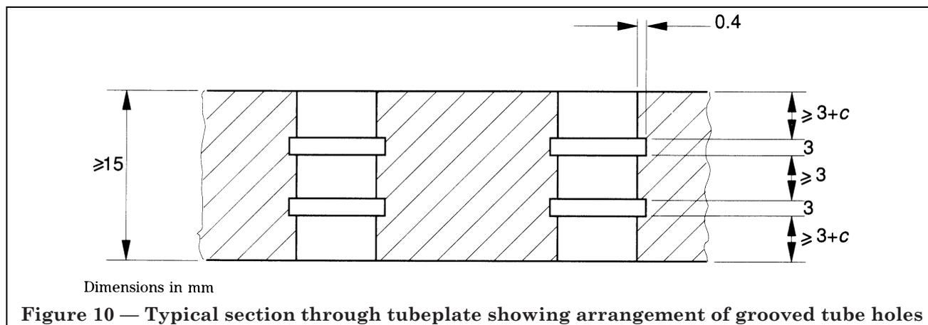
Figure 10 — Typical section through tubeplate showing arrangement of grooved tube holes
