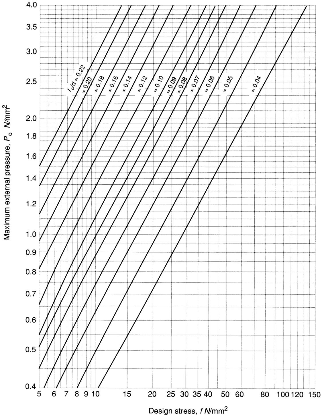
Figure 8 — Maximum external pressure of tubes for different ratios of  $t_c/d$
