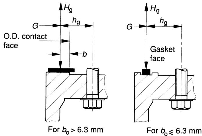
NOTE. The gasket seating width factors  $b_0$  and  $b$  shown apply only to flanged joints in which the gasket is contained entirely within the inner edges of the bolt holes.
