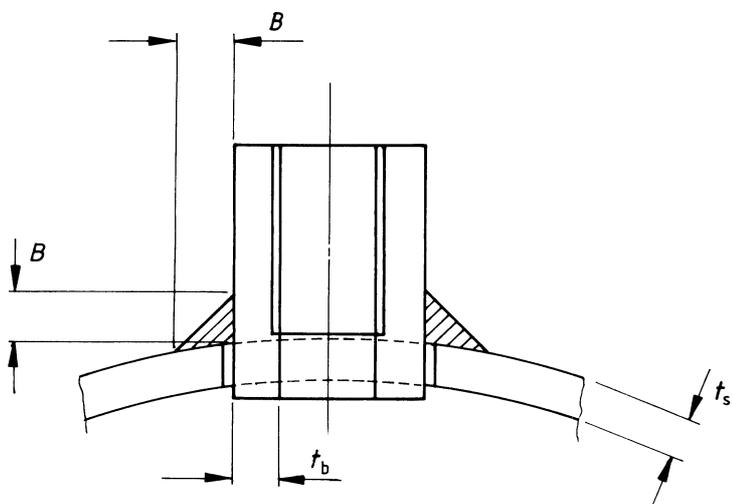
NOTE. Connection (c) is not recommended where the inside of the vessel is accessible for welding.
