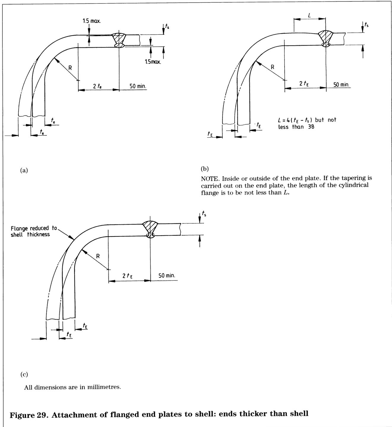
**Figure 29. Attachment of flanged end plates to shell: ends thicker than shell**
