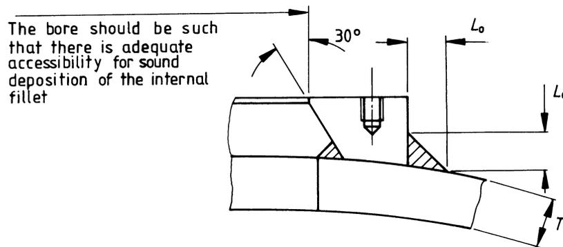
NOTE. The sizes of the fillet welds should be based on the loads transmitted, paying due regard to all fabrications and service requirements, but in any case should not be less than 6 mm.
