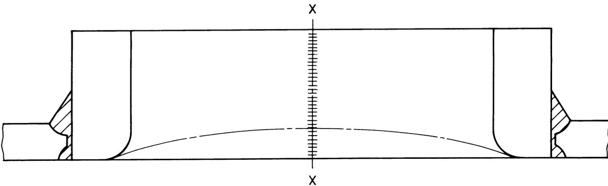
Alternative forging made in halves and fusion-welded along XX.
