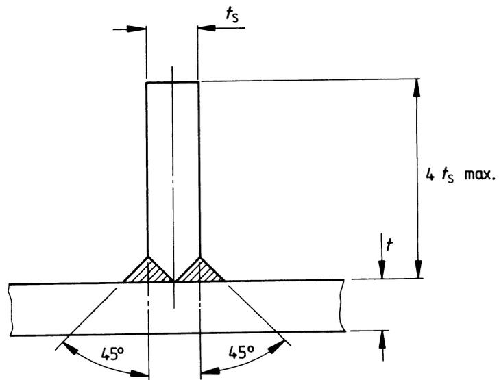
NOTE.  $t_s$  is to be equal to or greater than  $t$ , but not greater than  $2t$  and in no case to exceed 20 mm.
