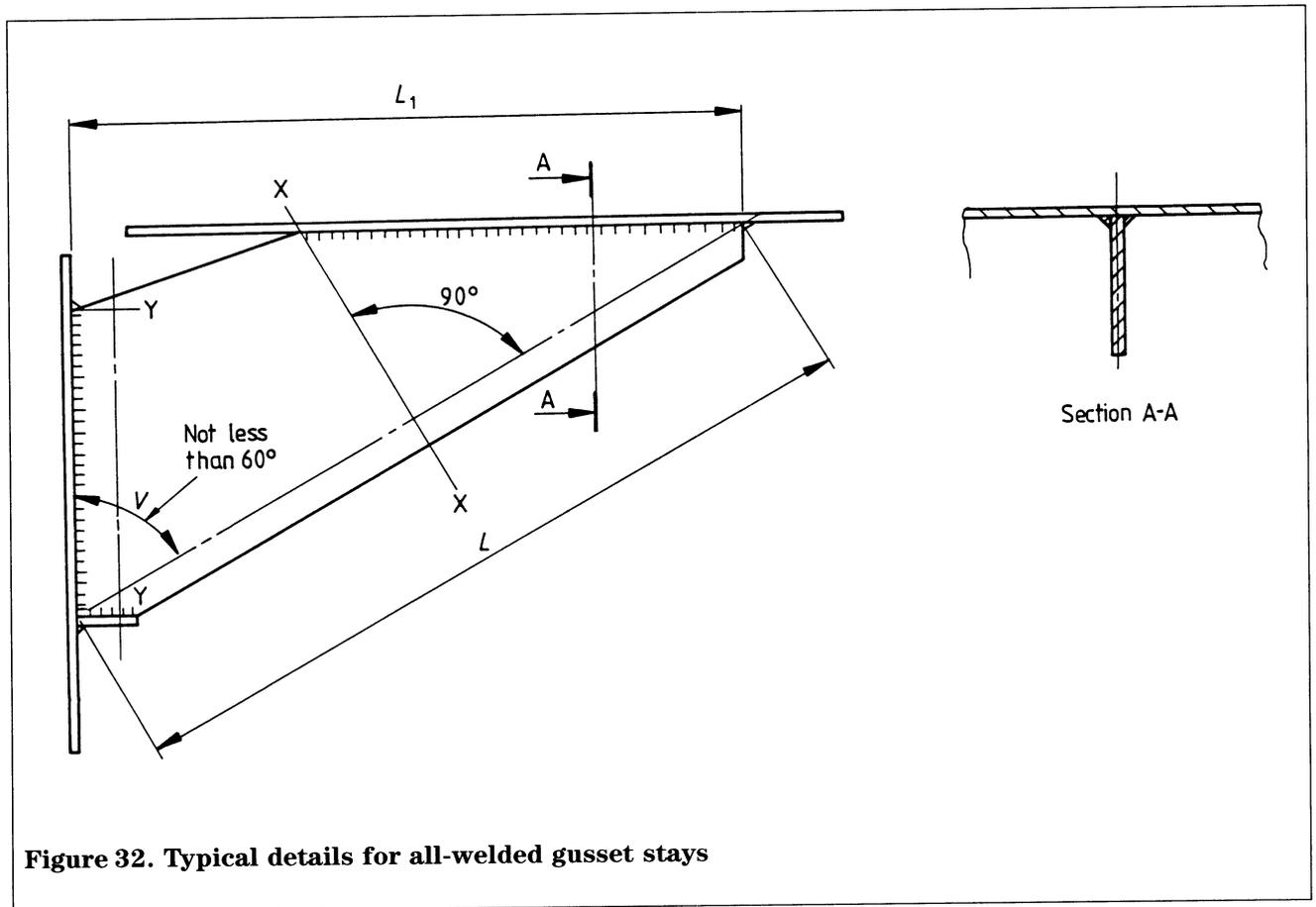
**Figure 32. Typical details for all-welded gusset stays**
