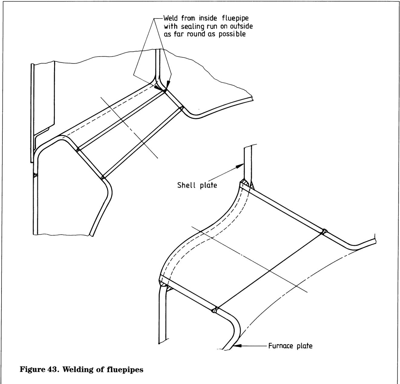
**Figure 43. Welding of fluepipes**
