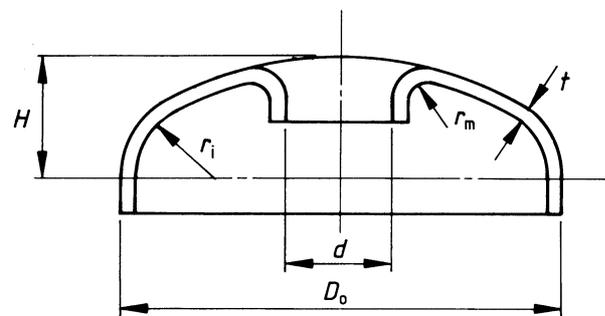
(c) End with manhole (semi-ellipsoidal or torispherical)
