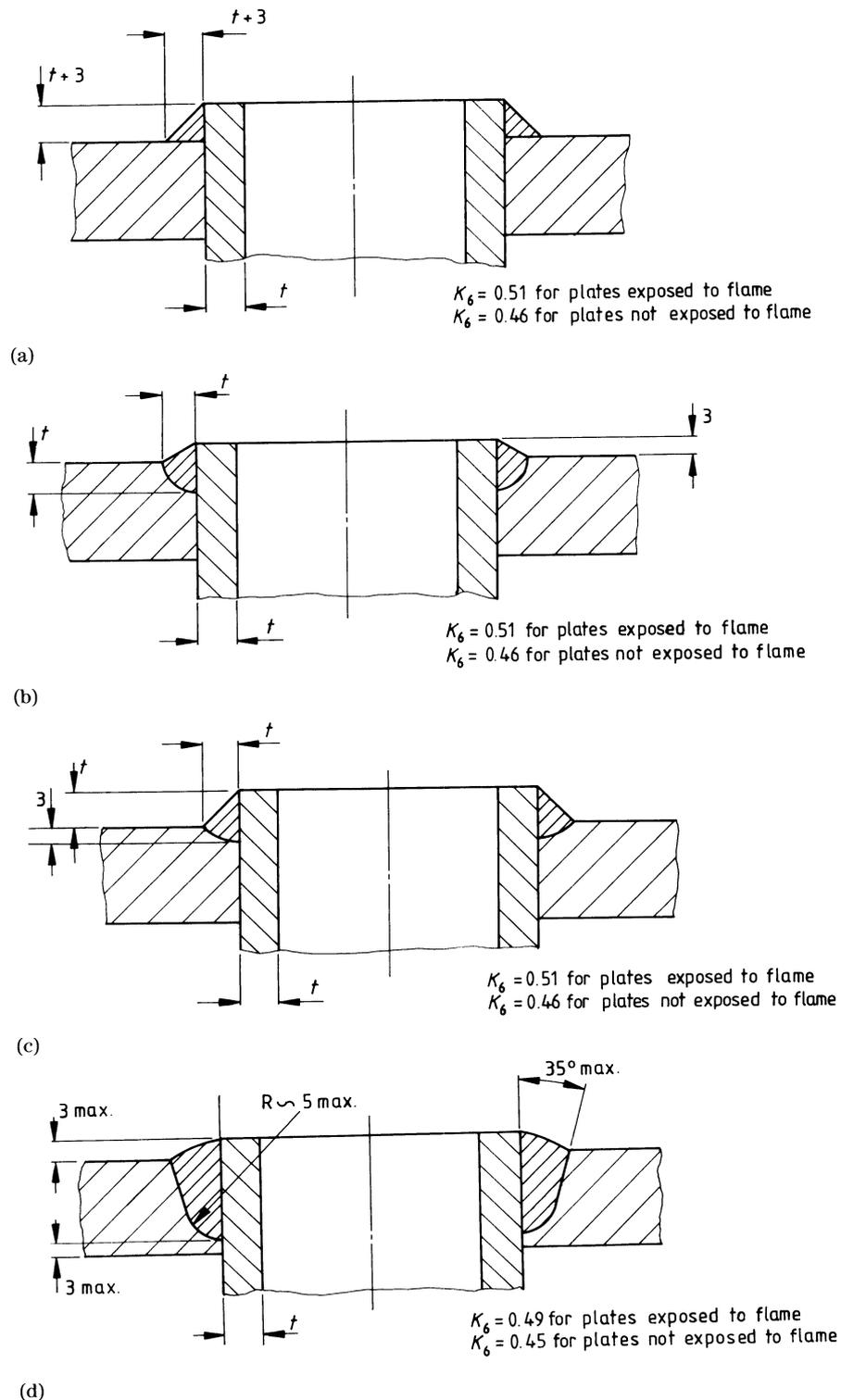
**Figure 34. Attachment of stay tubes to tube plates**
