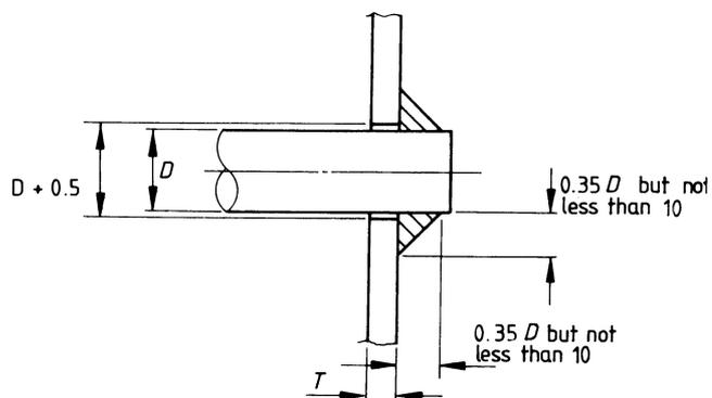
NOTE. Where these bar stays are exposed to flame or comparably high temperature, the stress on the stay is to be limited to  $52 \text{ N/mm}^2$  and the stay is not to project beyond the fillet weld.
