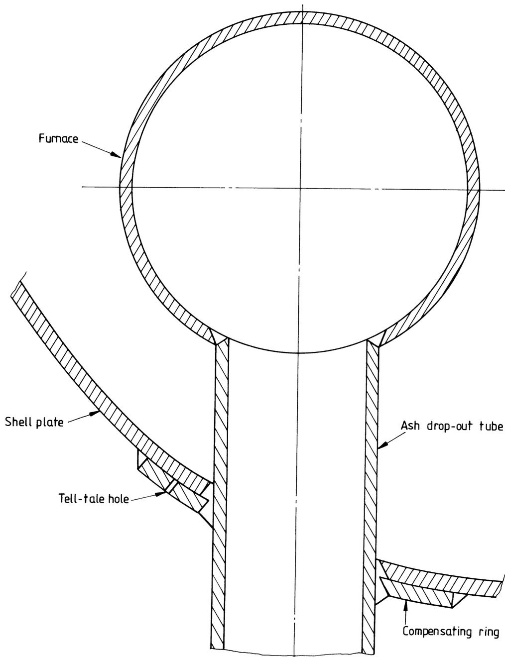
**Figure 4. Typical method of attachment of ash drop-out tube**
