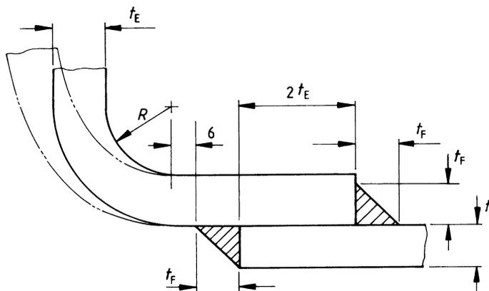
NOTE. The furnace to end plate attachment is suitable for front ends only, or in cases where there is no impingement of flame or hot gases.
