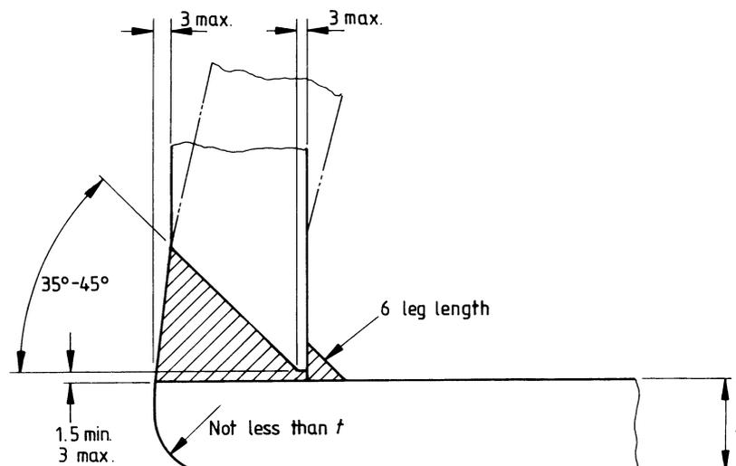
NOTE. The plate edge radius of not less than  $0.5 t$  is only required when the furnace end is exposed to a flame or comparatively high temperature, e.g. at the entry to the reversal chamber.
