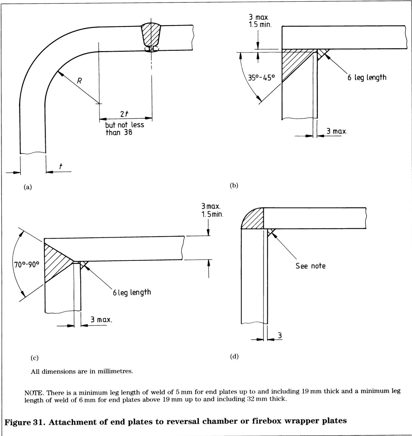
**Figure 31. Attachment of end plates to reversal chamber or firebox wrapper plates**
