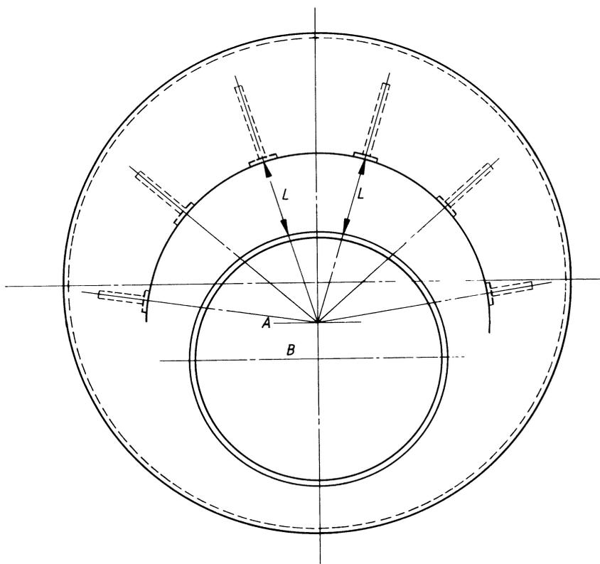
NOTE. The distance A - B between the centre of the stay circle and centre of furnace is not to be less than  $3t + 63$ , where  $t$  is the thickness of the end plate (in mm).
