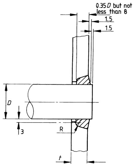
NOTE. This form of attachment is also suitable for longitudinal bar stays.
