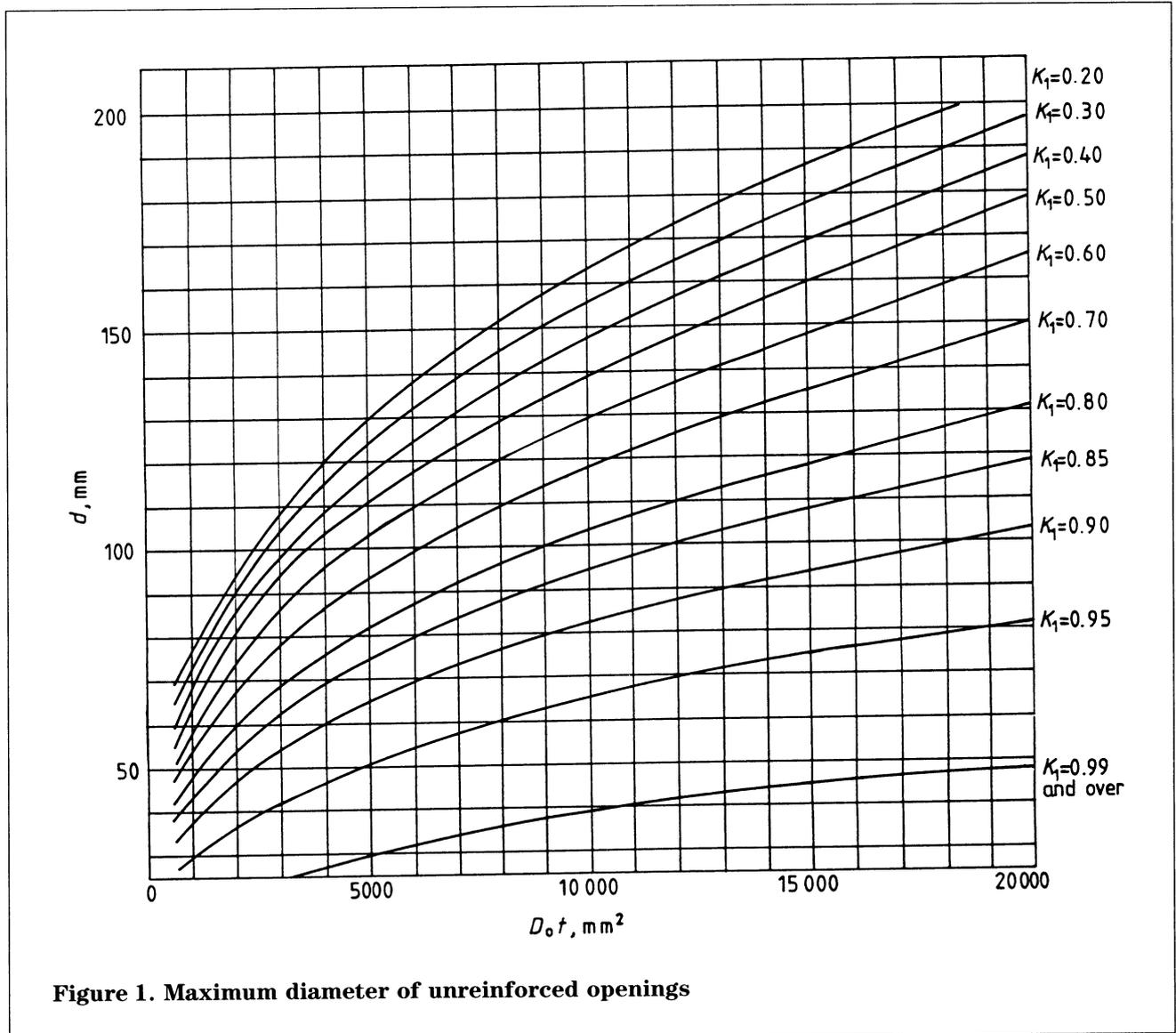
Figure 1. Maximum diameter of unreinforced openings
