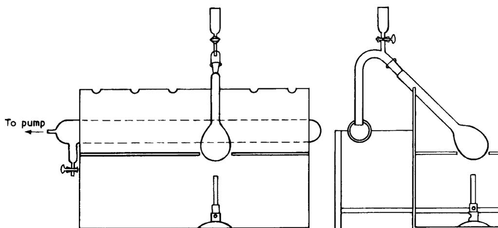
Figure 1 — Apparatus for the wet oxidation of the sample
