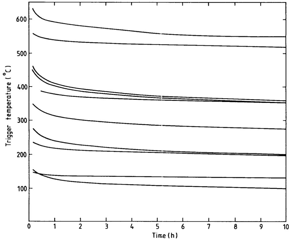
Figure 4 — Examples of trigger temperature-time relationships for some single-change paints
