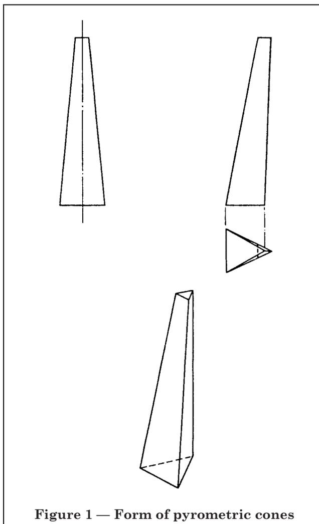
Figure 1 — Form of pyrometric cones
