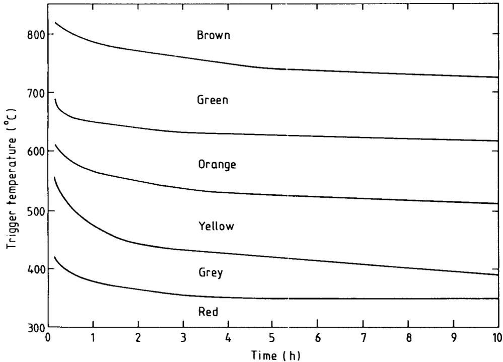
Figure 5 — Examples of trigger temperature-time relationships for a multi-change paint
