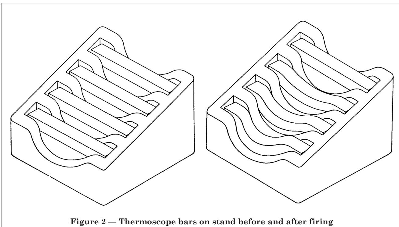
Figure 2 — Thermoscope bars on stand before and after firing
