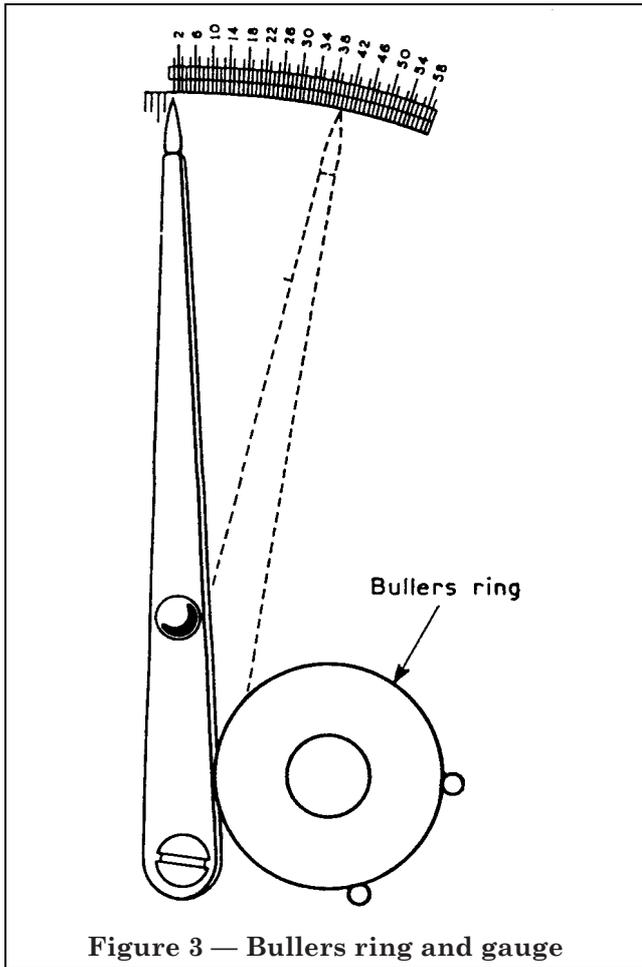
Figure 3 — Bullers ring and gauge
