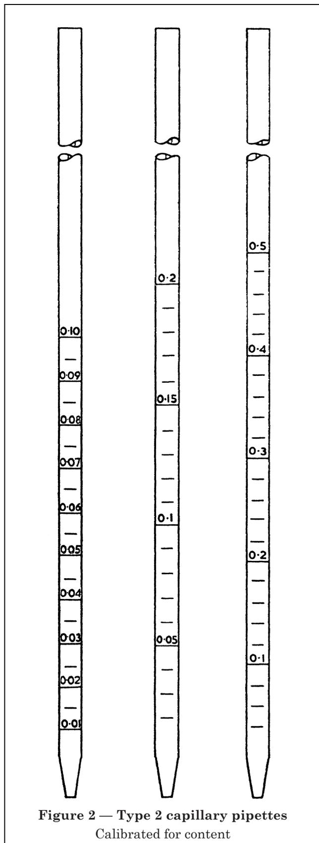
Figure 2 — Type 2 capillary pipettes
