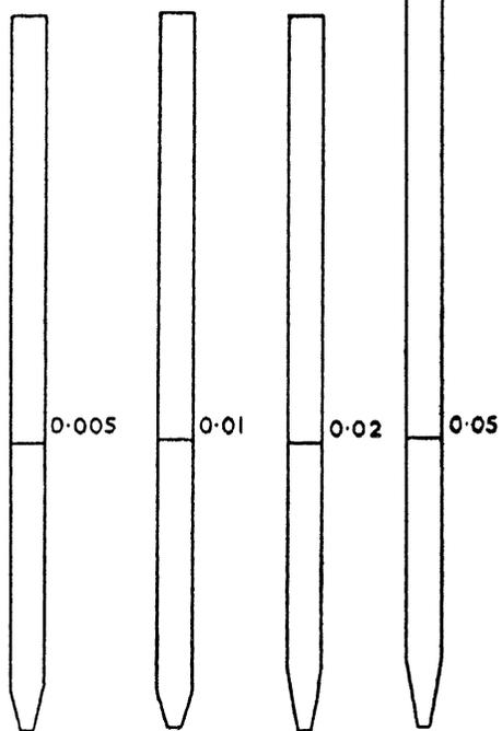
**Figure 3 — Type 3 capillary pipettes**
