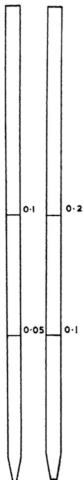
**Figure 4 — Type 4 capillary pipettes**
