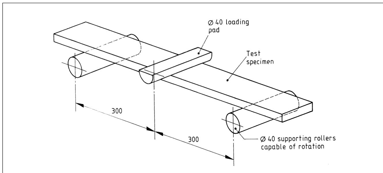
All rollers, radiused loading pads or blocks shall be manufactured from steel and shall have a circular cross-section with a diameter of  $40 \text{ mm} \pm 2 \text{ mm}$ ; they shall be at least 10 mm longer than the width of the test specimen.
