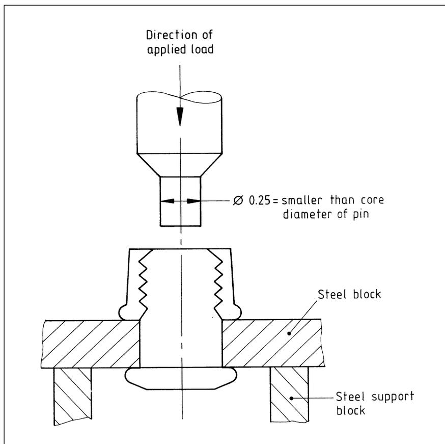
Figure B.2 Pull-out test arrangement
