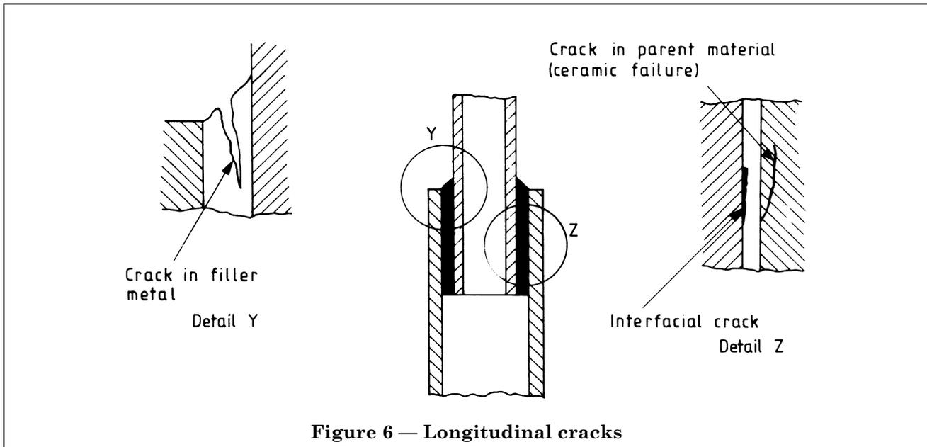
**Figure 6 — Longitudinal cracks**
