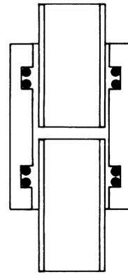
The use of loading grooves ensures that the filler metal is in the correct position
