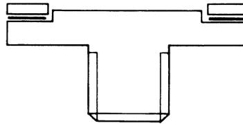
When the filler metal is pre-placed in the joint, washers may be preferred to wire rings since there is less displacement of the components
