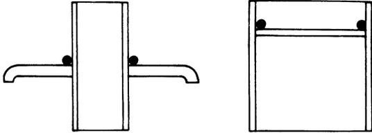
Rings are suitable for a wide range of tube/plate and tube/fitting assemblies
