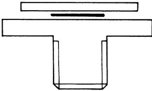
Brazing foil discs and shims are widely used for joining flat surfaces
