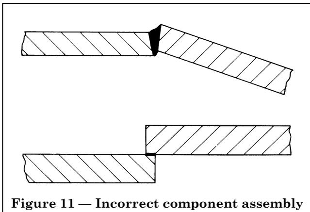
Figure 11 — Incorrect component assembly
