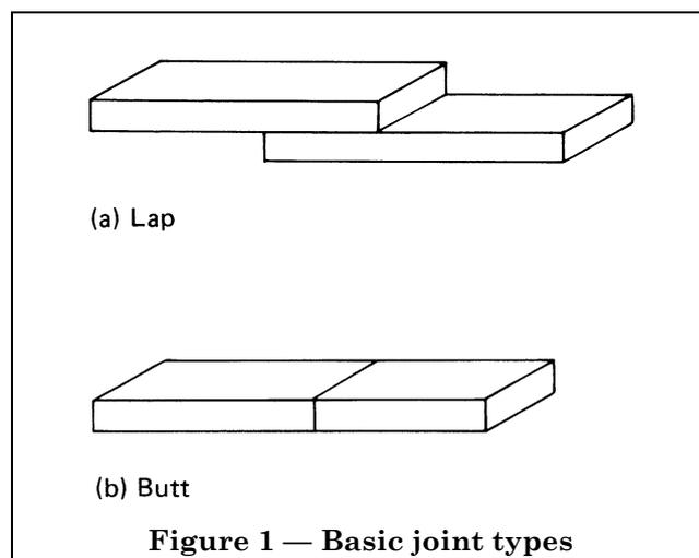
Figure 1 — Basic joint types
