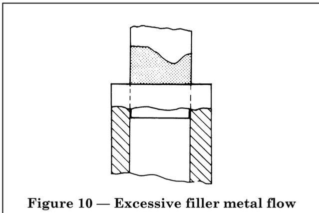
Figure 10 — Excessive filler metal flow
