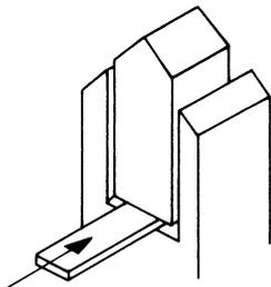
Cut lengths of wire, or strip often prove a convenient method of pre-placing filler metal
