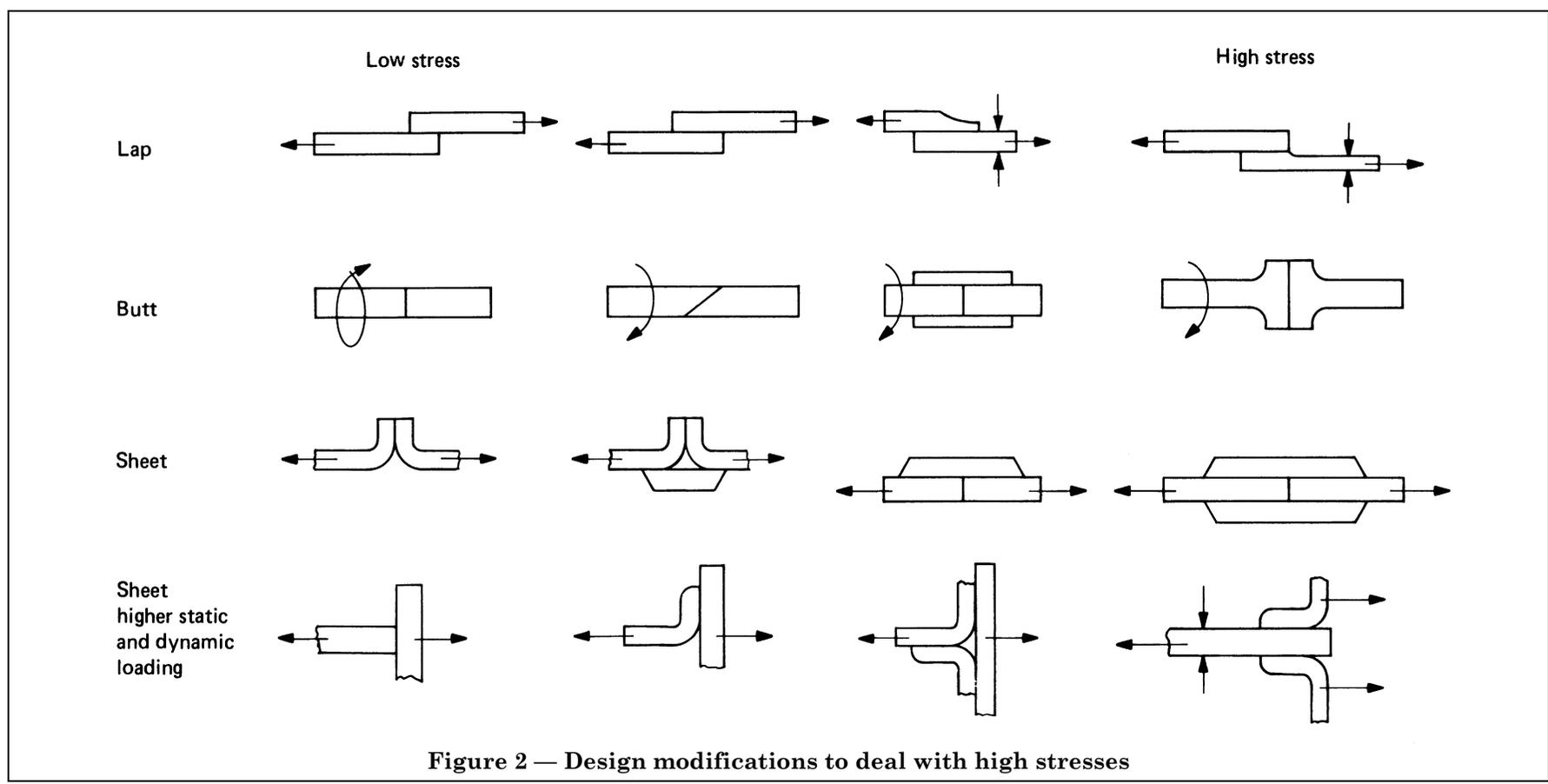
Figure 2 — Design modifications to deal with high stresses
