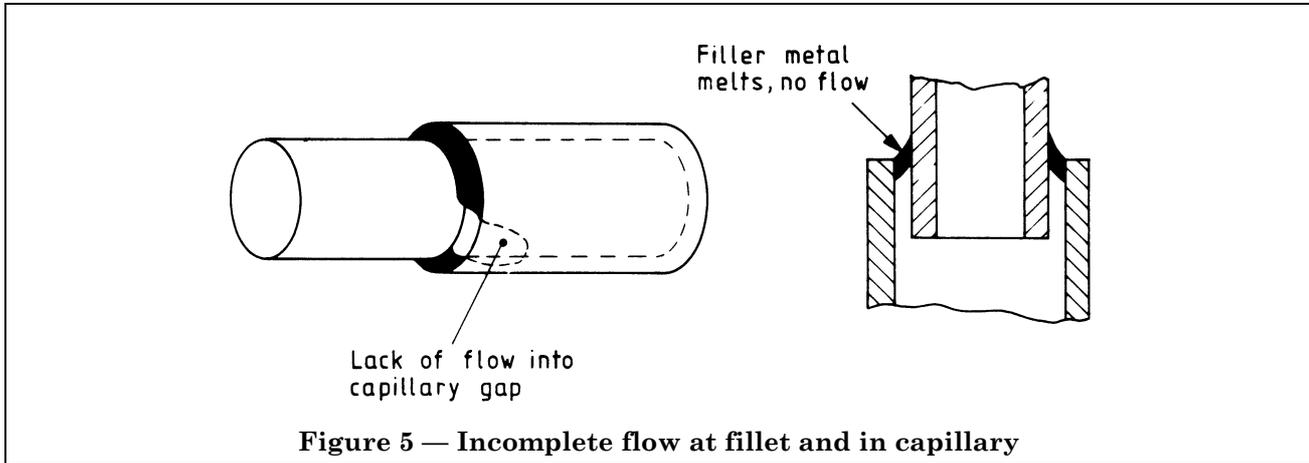
**Figure 5 — Incomplete flow at fillet and in capillary**
