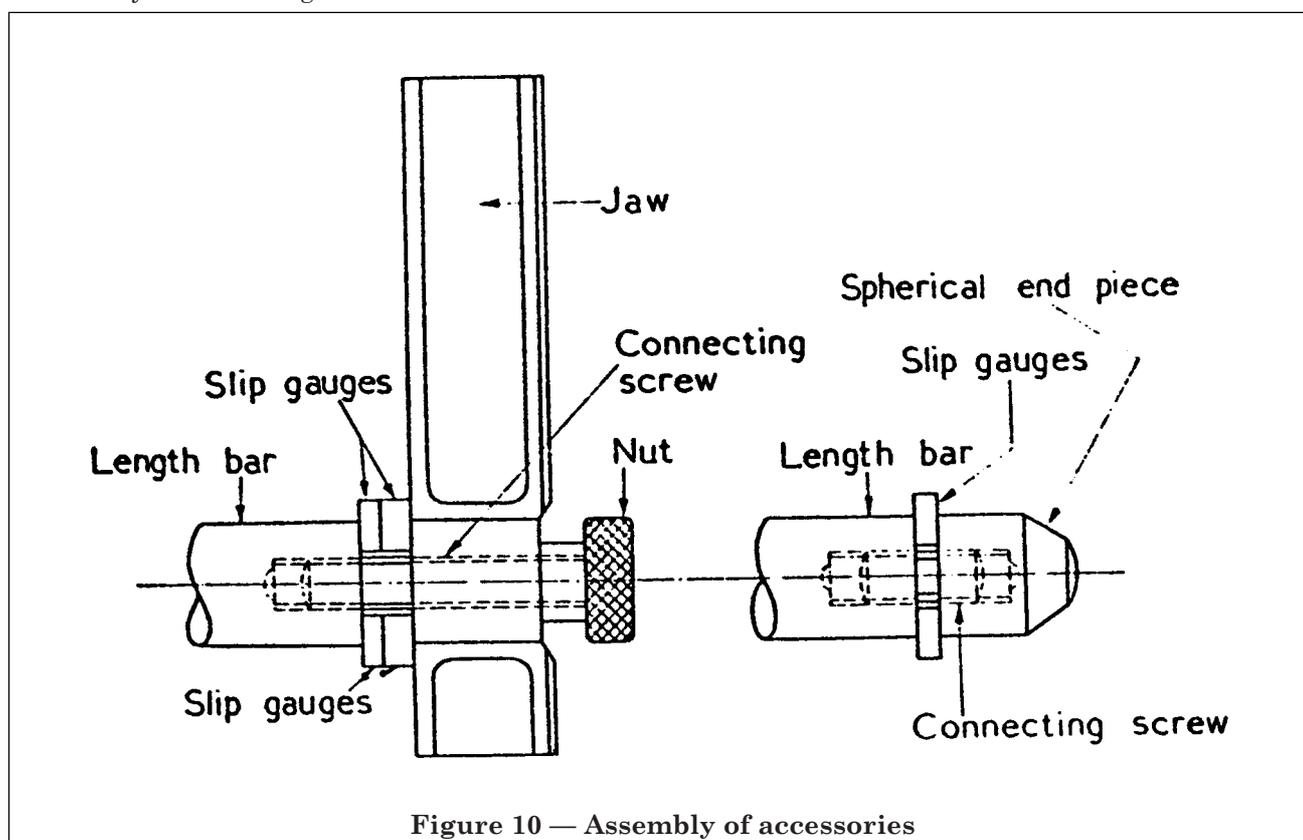
Figure 10 — Assembly of accessories
