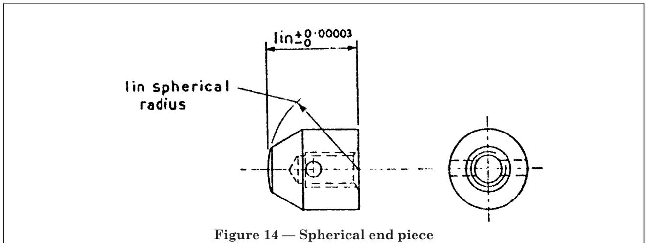
Figure 14 — Spherical end piece
