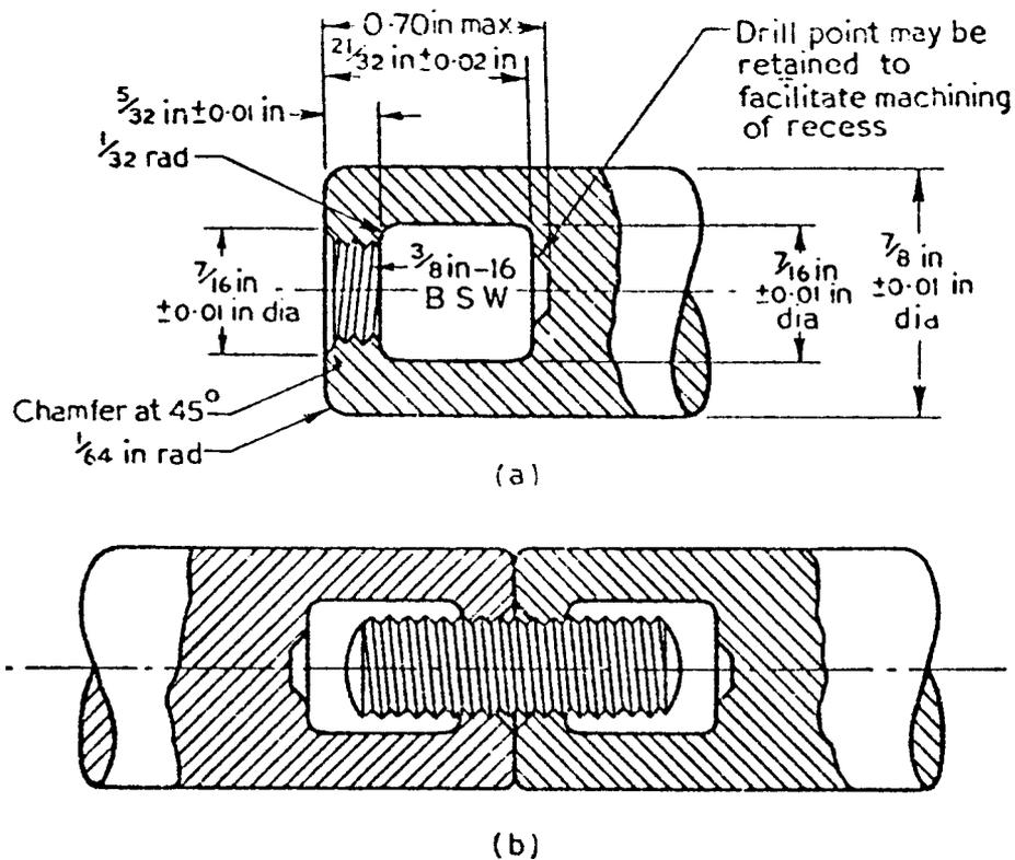
**Figure 8 — New design of threaded connection for length bars**
