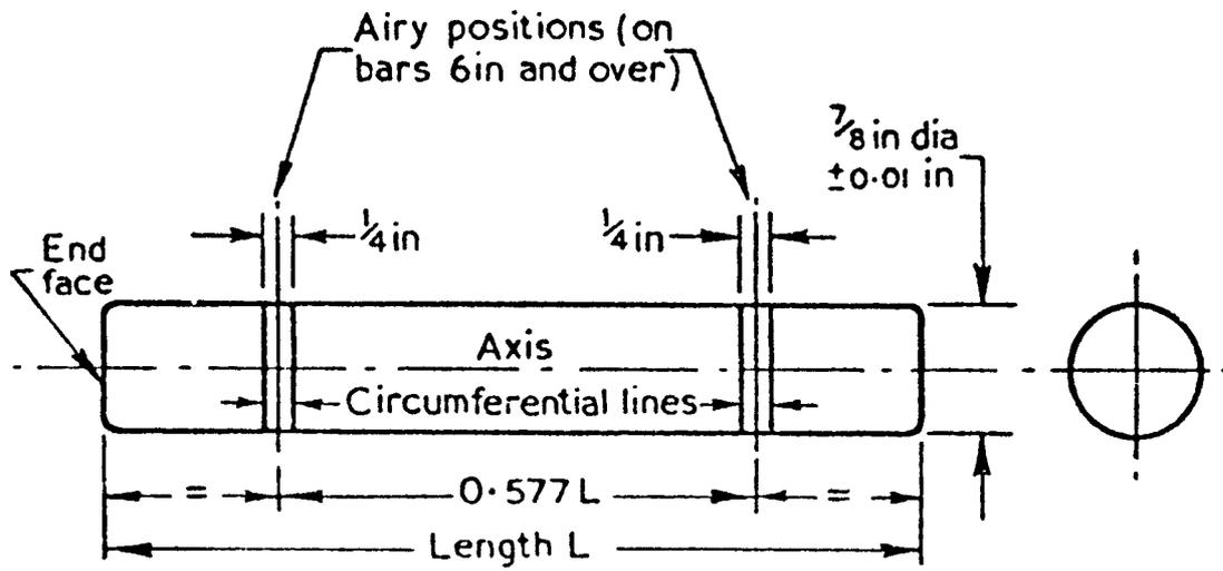
Figure 5 — Reference or calibration grade length bar
