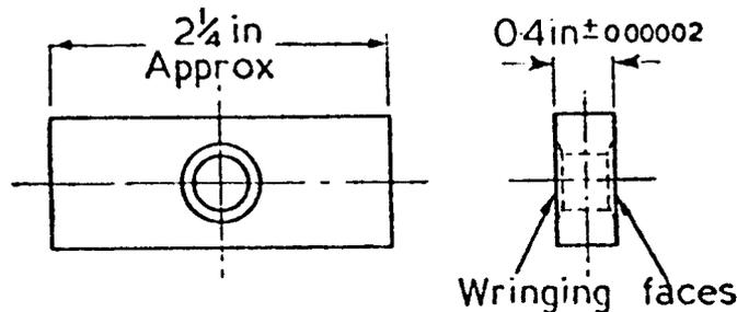
Figure 13 — Small plane-faced jaw
