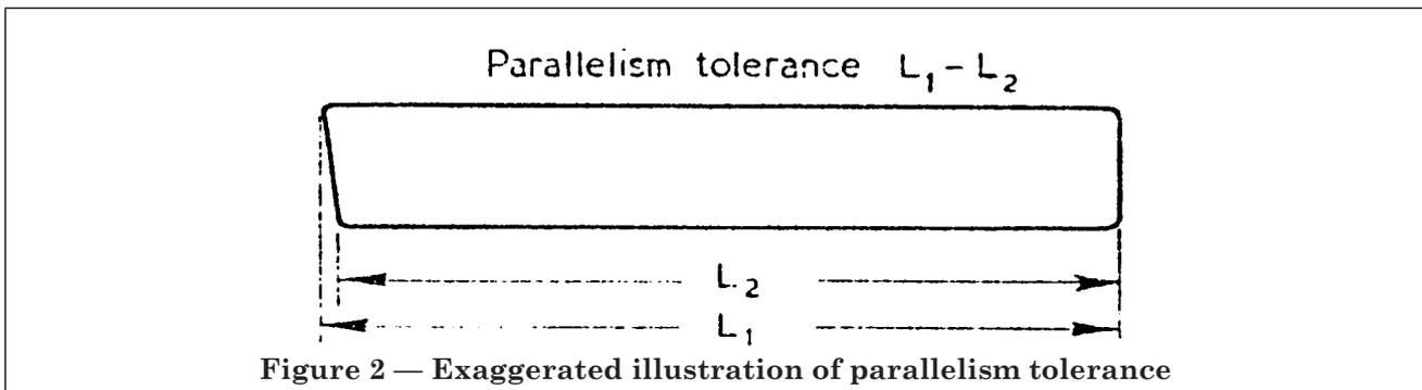
Figure 2 — Exaggerated illustration of parallelism tolerance
