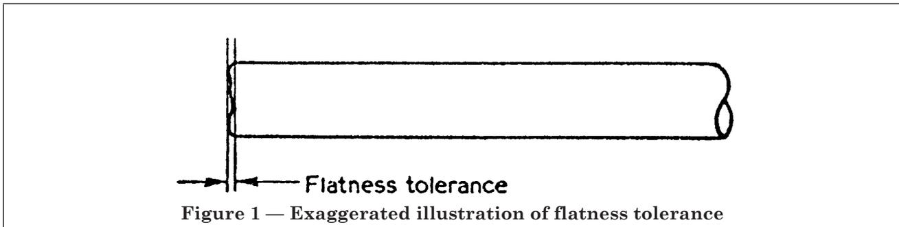
Figure 1 — Exaggerated illustration of flatness tolerance
