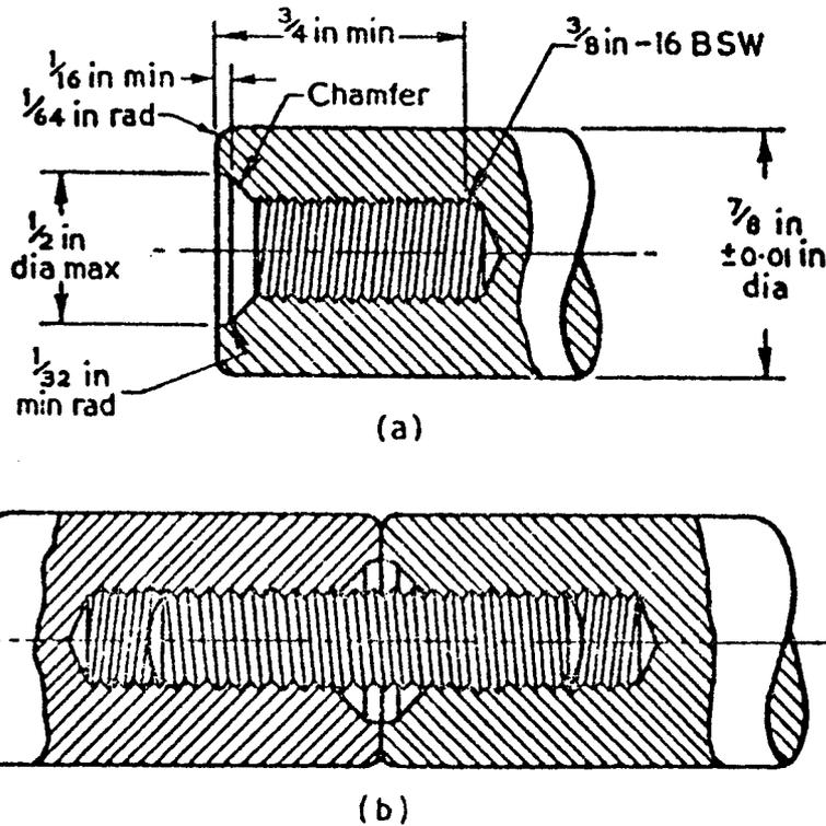
Figure 9 — Original type of screwed connection for length bars
