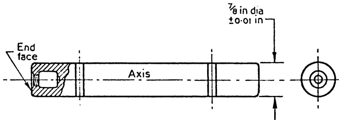
Figure 6 — Inspection grade length bar
