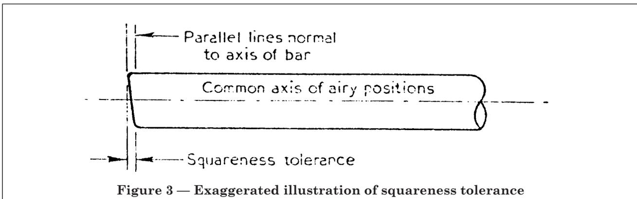
Figure 3 — Exaggerated illustration of squareness tolerance
