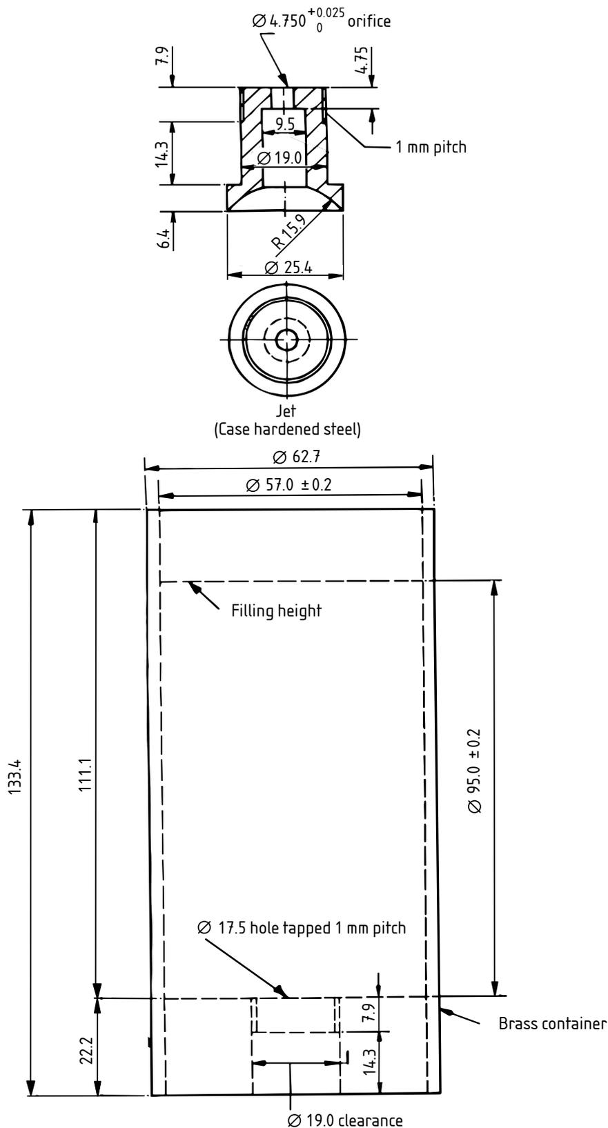
Figure A.3 — Container for compound and jet
