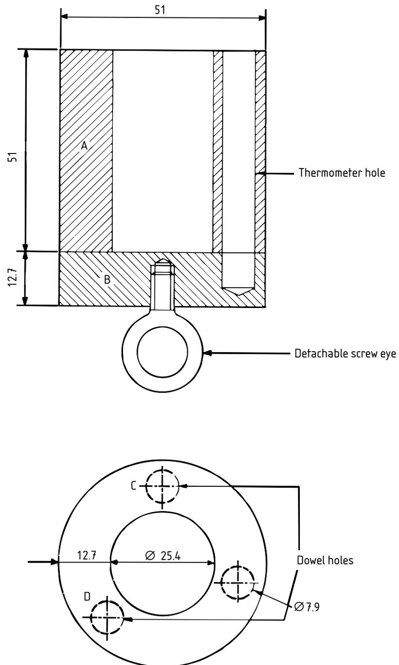
**Figure D.1 — Apparatus for determination of adhesive properties**
