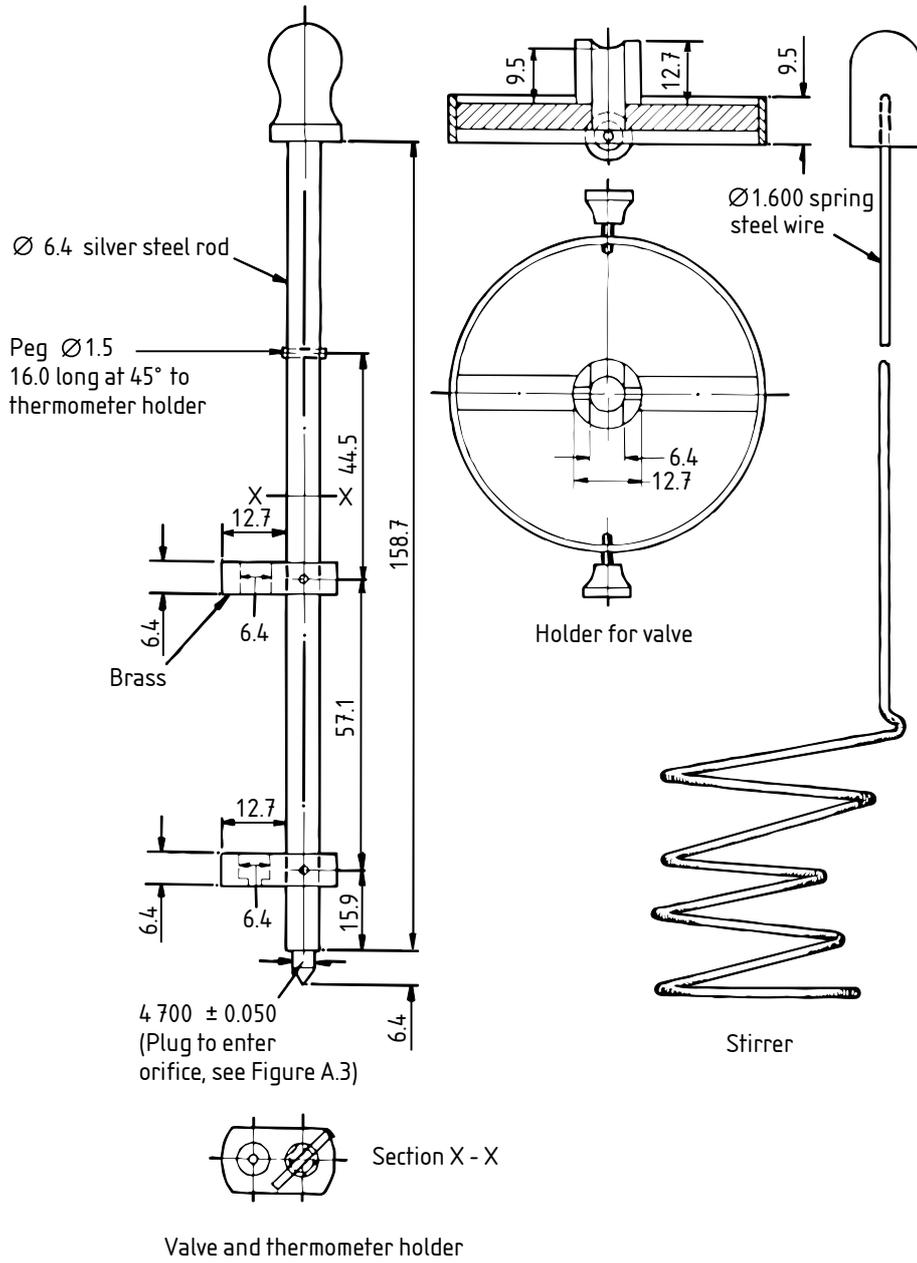
Figure A.2 — Valve, holder and stirrer
