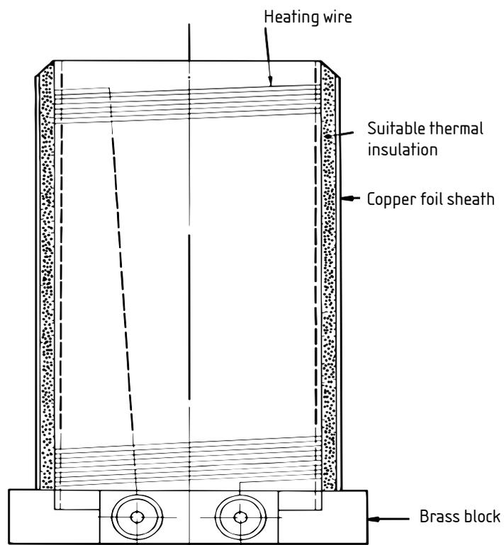
Figure A.4 — Outer vessel for electrical heating
