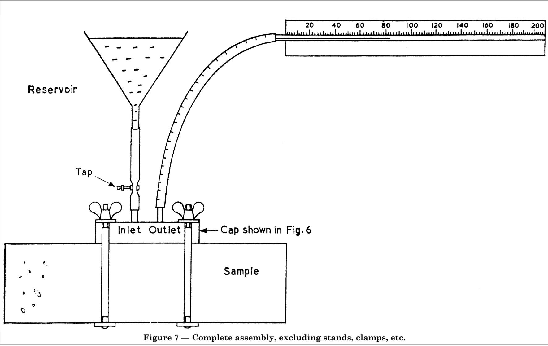
Figure 7 — Complete assembly, excluding stands, clamps, etc.
