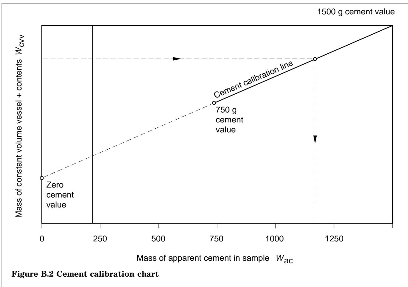
Figure B.2 Cement calibration chart
