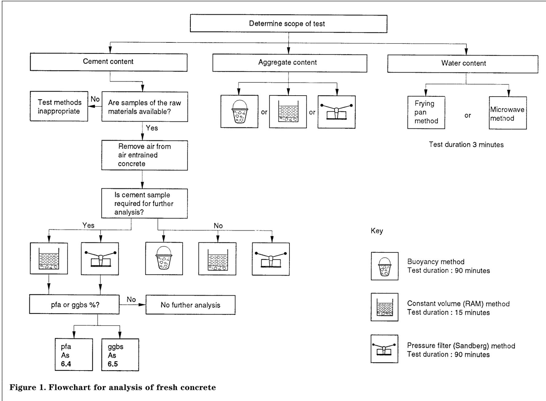
Figure 1. Flowchart for analysis of fresh concrete
