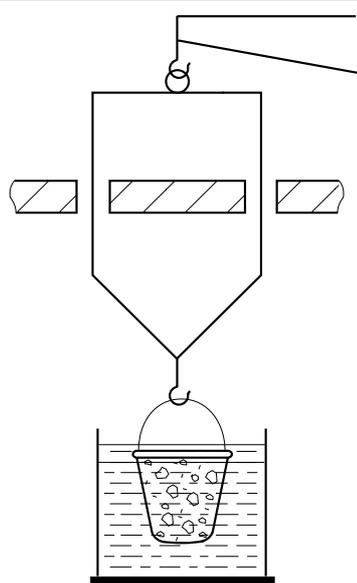
a) Typical balance and support methods
