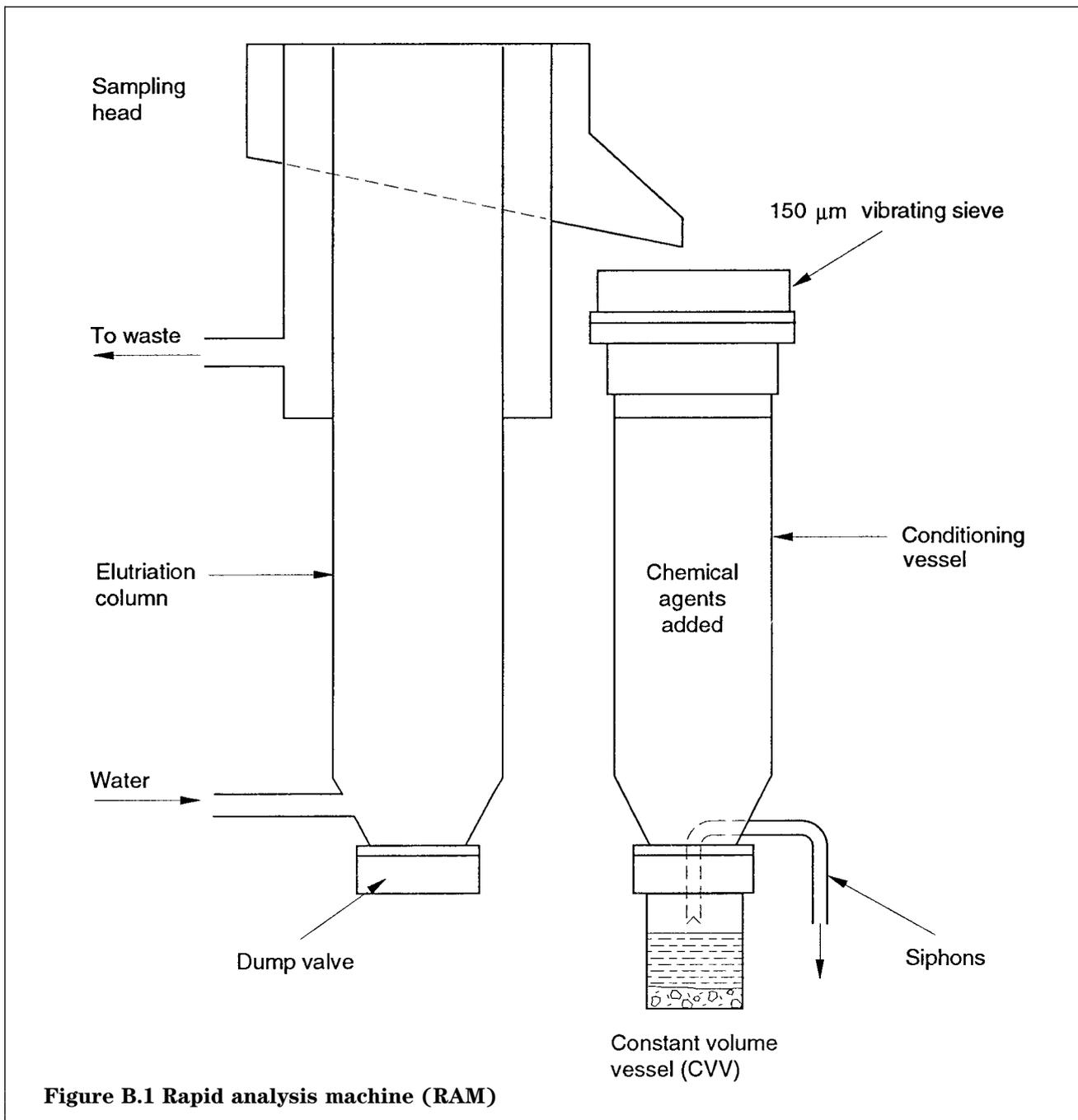
Figure B.1 Rapid analysis machine (RAM)
