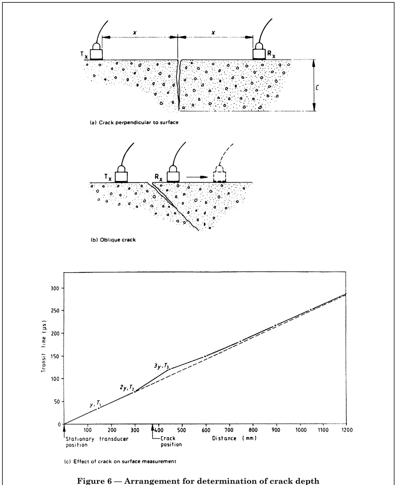
Figure 6 — Arrangement for determination of crack depth
