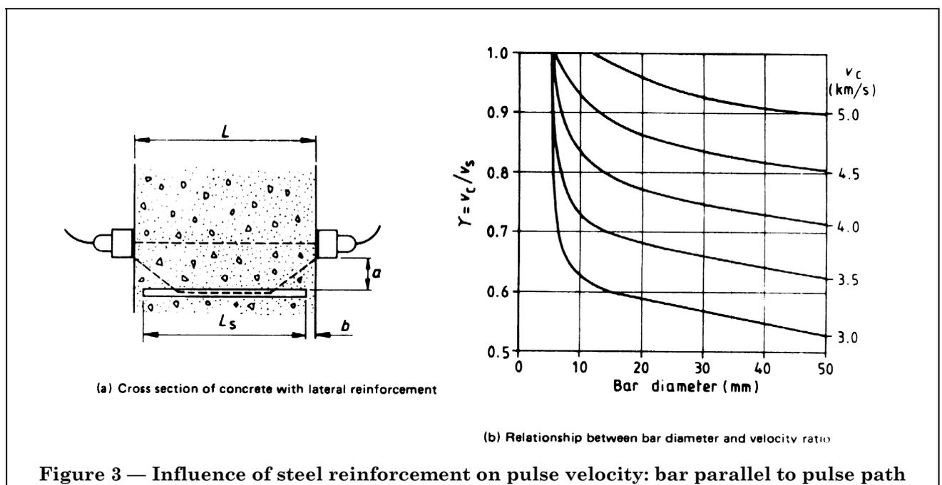
Figure 3 — Influence of steel reinforcement on pulse velocity: bar parallel to pulse path
