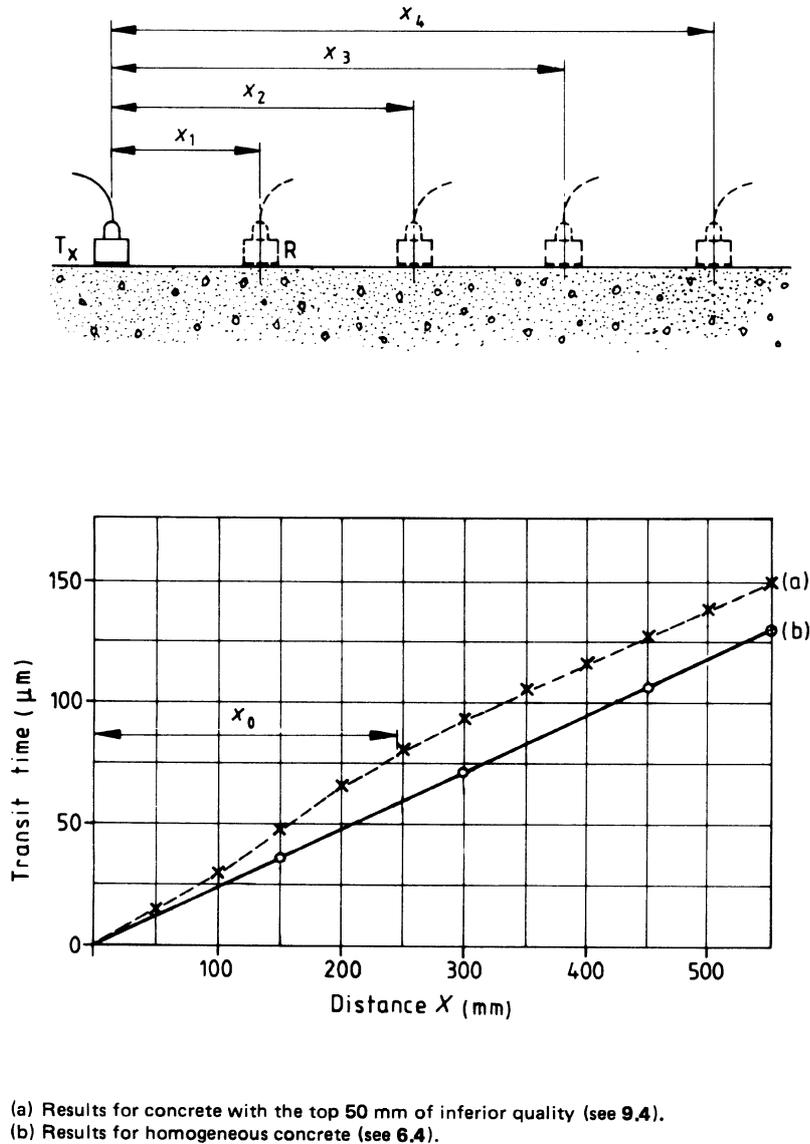
Figure 2 — Pulse velocity determination by indirect (surface) transmission
