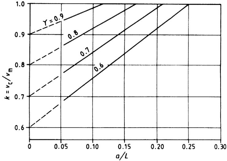
Figure 4 — Influence of steel reinforcement on pulse velocity: correction factors for bars parallel to pulse path ( $a > 2 b$ ) [see Figure 3 a)]
