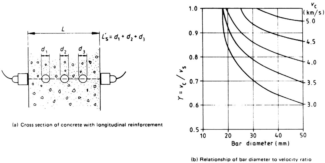
Figure 5 — Influence of steel reinforcement on pulse velocity: bars normal to pulse path
