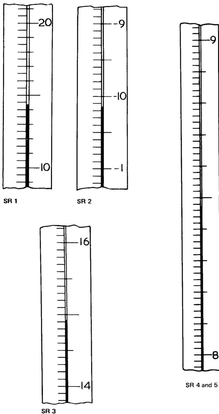
Figure 2 — Examples of graduation and figuring for secondary reference thermometers (continued)
