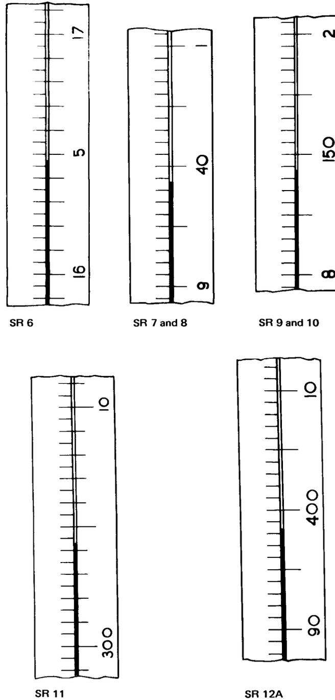
Figure 2 — Examples of graduation and figuring for secondary reference thermometers (*concluded*)
