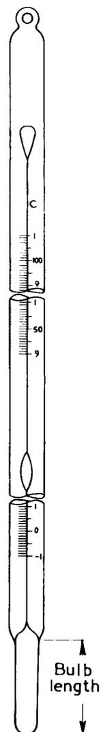
Figure 1 — Typical construction of a thermometer
