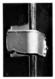
(c) No Cracking or Adhesive Failure
