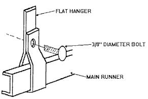
FIG. 9 Flat Hanger Attached to Main Runner Using Bolt
