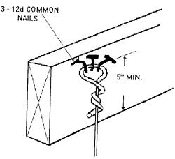
FIG. 6 Wire Hanger Attached to Wood Member Using Nails
