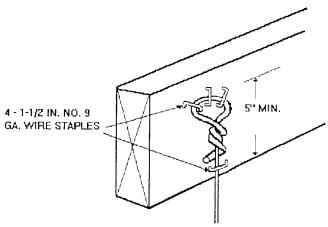
FIG. 7 Wire Hanger Attached to Wood Member Using Staples
