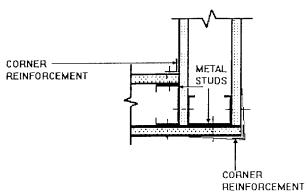
FIG. 2 Partition Corner Detail
