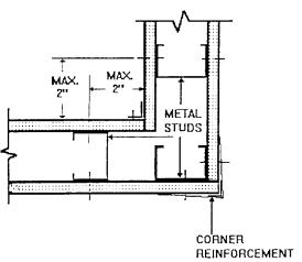
FIG. 3 Partition Corner Detail
