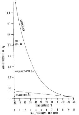
FIG. X1.3 Limiting Vapor Pressure Gradient Plot (14)
