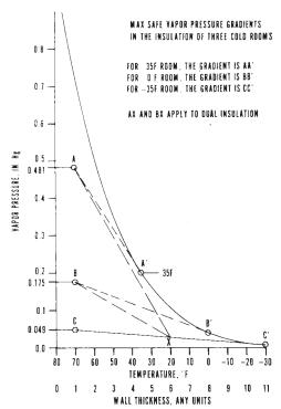
FIG. X1.4 Saturation Vapor Pressure vs. Temperature (14)
