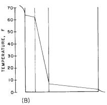
FIG. X1.1 Vapor Pressure and Temperature Gradients of Building Wall (6)
