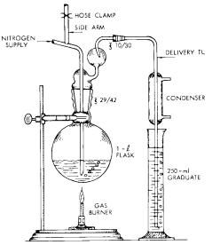
FIG. 7 Apparatus for Distillation of Chlorine
