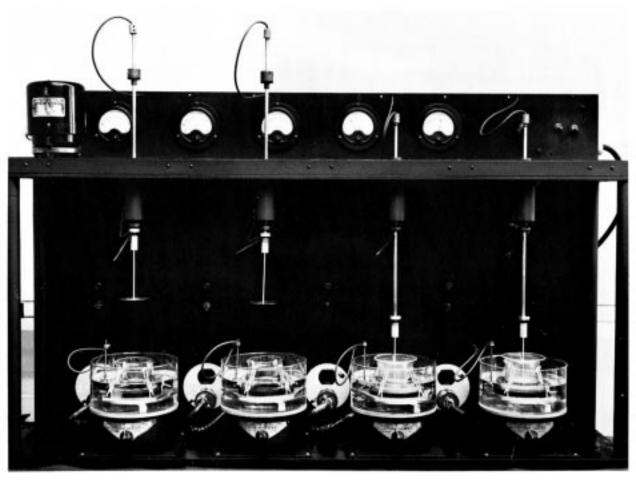
FIG. 10 Multiple-Cell Electroplating Apparatus
