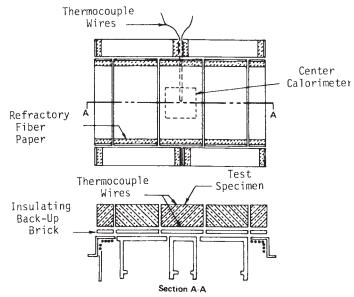
FIG. 1 Arrangement of Refractory-Fiber Paper Strips in Calorimeter Assemblage
