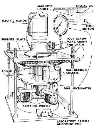
FIG. 2 Dressing Wheel Abrasion Test Machine
