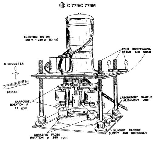
FIG. 1 Revolving Disks Abrasion Test Machine
