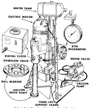
FIG. 3 Ball Bearing Abrasion Test Machine
