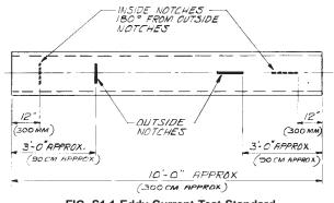
FIG. S1.1 Eddy-Current Test Standard
