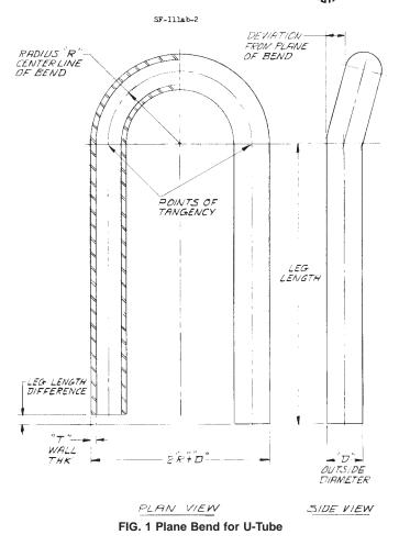
A 1016M. Those tolerances do not apply to the bent portion of the U-tubes. At the bent portion of a U-tube for  $R = 2 \times D$  or greater, neither the major nor minor diameter of the tube shall deviate from the nominal diameter prior to bending by more than 10 %. If less than  $2 \times D$  is specified, tolerances could be greater.
