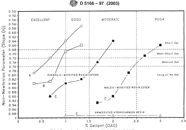
FIG. 1 Determination of Lithographic Ink Resin Gelability
