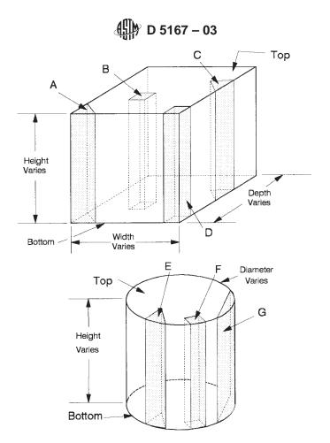
A,B,C,D,E,F & G are several typical vertical samples that can be taken from the manufacturer's original shipped sealant units.
