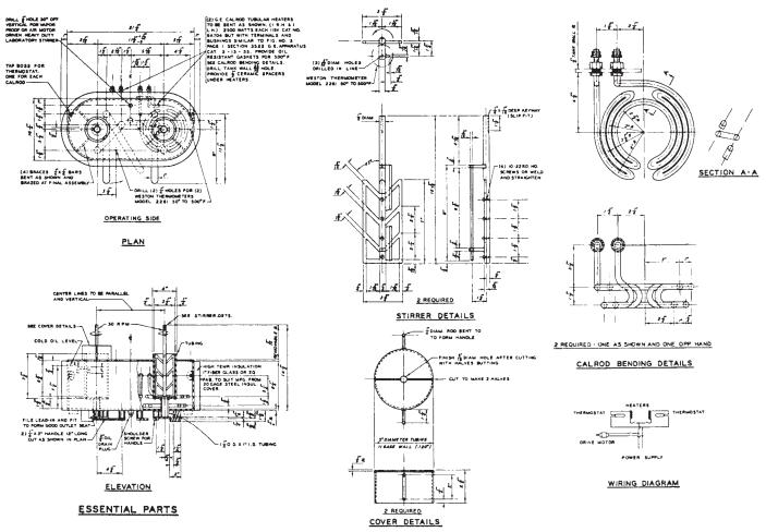
FIG. 2 Detailed Drawing of Joint Sealant Laboratory Melting Unit
