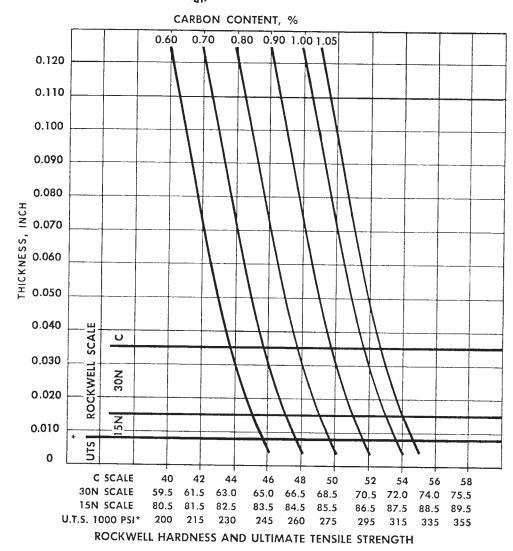
Note 1—For thicknesses less than 0.008 in. [0.20 mm] use of the tension test is recommended.
