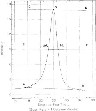
FIG. 1 Typical Diffraction Scan of Petroleum Coke
