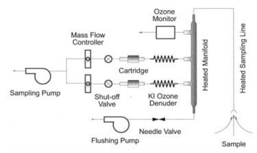
FIG. 3 A Dual-Cartridge Sampling System with Heated Manifold for Carbonyl Compounds in Ambient Air
