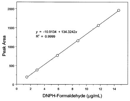
FIG. 9 Example Calibration Curve for Formaldehyde
