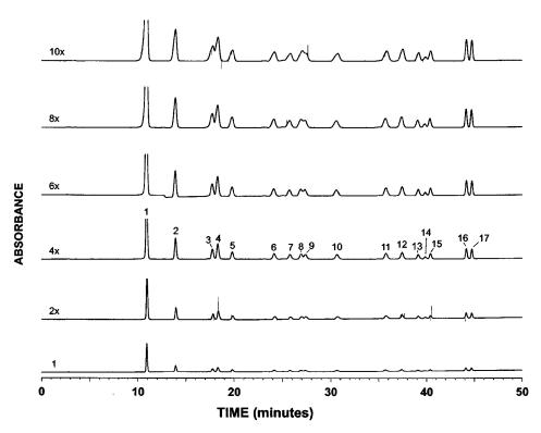
FIG. 8 Typical Six-Level Multiple-Component Standard Calibration Chromatogram
