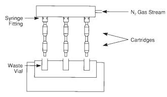
(b) Rack for Drying DNPH-Coated Cartridges
