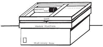
FIG. 2 Aerosol Can on Eberbach Shaker
