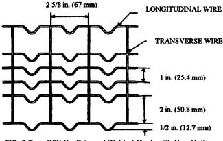
FIG. 3 Type WW-N—Crimped Welded Mesh with Non-Uniform Longitudinal Wire Spacing
