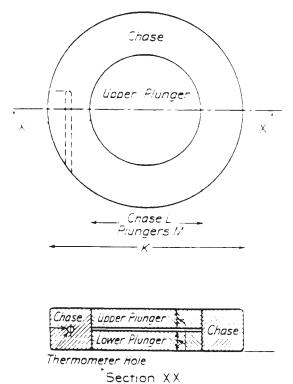
FIG. 2 Compression Mold for Disk Test Specimens
