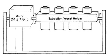
FIG. 2 Rotary Agitation Apparatus
