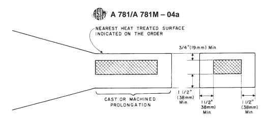
Note—Longitudinal axis and gage length of test specimen must be within cross-hatched zone. FIG. 6 Prolongation Test Specimen
