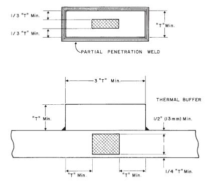
NOTE—Longitudinal axis and gage length of test specimen must be within cross-hatched zone. FIG. 7 Thermal Buffer Pad
