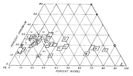
NOTE 1—The approximate areas of microstructures to be expected at room temperature are indicated as follows: I—Martensite
