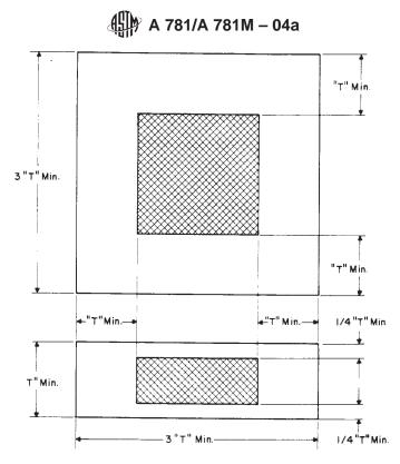
Note—Longitudinal axis and gage length of test specimen must be within cross-hatched zone. FIG. 5 Separately Cast Block
