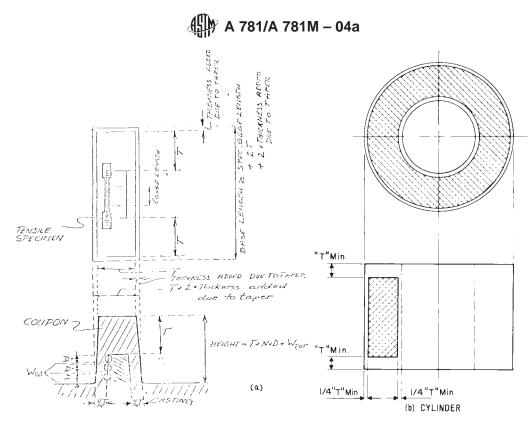
Minimum length of the base—Specimen gage length + 2xT + 2x the thickness due to the tapes. Minimum width of the base—T + 2x the thickness added due to the taper.
