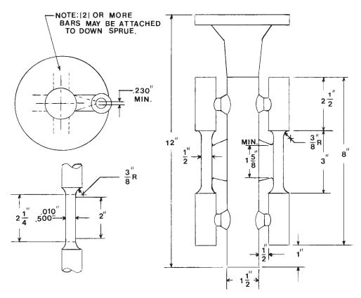
Note—Coupons produced in this manner are suitable for austenitic alloys only. The mold may be preheated for pouring to produce a sound coupon. FIG. 3 Cast-To-Shape Test Coupon for Tension Specimen
