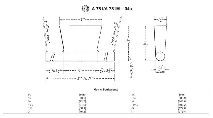
NOTE—Pour through head; cover molten head with powdered charcoal, coke dust, and so forth, immediately after pouring, in order to keep head fluid as long as possible.
