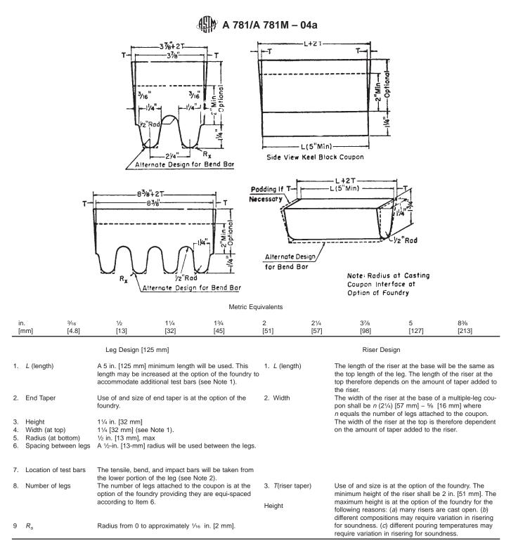
NOTE 1—Test Coupons for Large and Heavy Steel Castings: The test coupons in Fig. 1 are to be used for large and heavy steel castings. However, at the option of the foundry the cross-sectional area and length of the standard coupon may be increased as desired.
