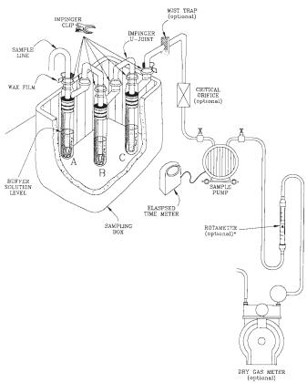
FIG. 1 Diagram of a Sampling Train and Sampling Apparatus
