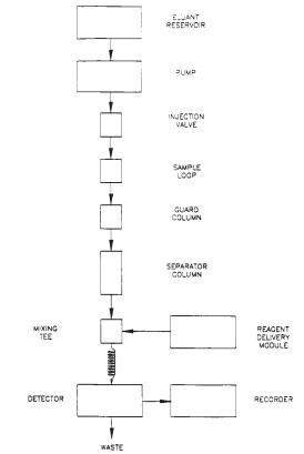
FIG. 2 Diagram of an Ion Chromatograph Using Post-Column Reagent Addition and Photometric Detection
