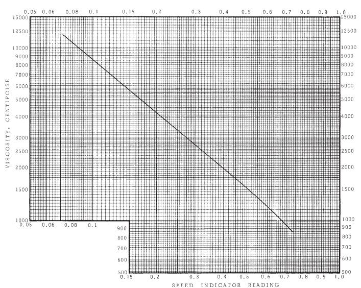
FIG. 4 Linearized Calibration Chart, Cold Cranking Simulator
