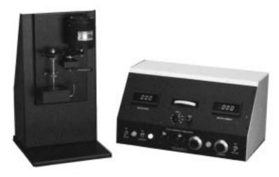
FIG. 1 Cold Cranking Simulator
