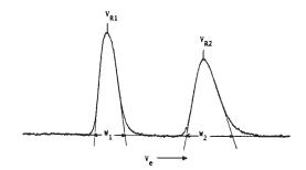
FIG. 3 Determination of Resolution,  $R_s$ , Using Narrow MWD Polystyrene Standards  $M_1 > M_2$
