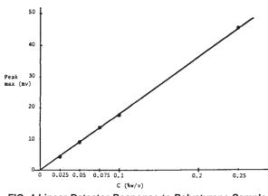
FIG. 4 Linear Detector Response to Polystyrene Sample Concentration
