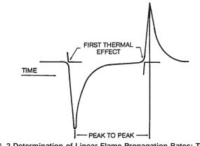
FIG. 2 Determination of Linear Flame Propagation Rates: Typical Stripchart Record
