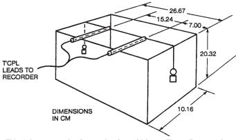
FIG. 1 Apparatus for Determination of Linear Flame Propagation Rates
