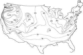
FIG. 1 Isoline Map of the Freeze-Thaw Severity Index
