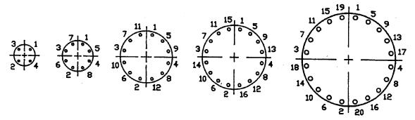
FIG. 3 Bolt Torquing Sequence
