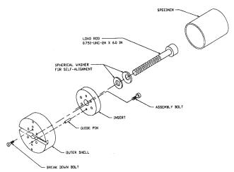
FIG. 1 Assembly Drawing for Tension Fixture and Specimen
