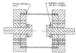
FIG. 7 Illustration of Assembled Tension Fixture and Specimen
