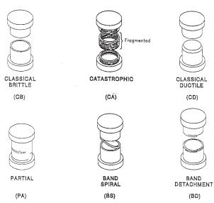
FIG. 8 Failure Modes for Hoop Wound Tubes in Tension
