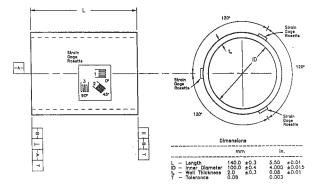
Note 1—Tube may be fabricated on a tapered mandrel with maximum taper of 0.0005 in./in. (0.0005 mm/mm) on the diameter.
