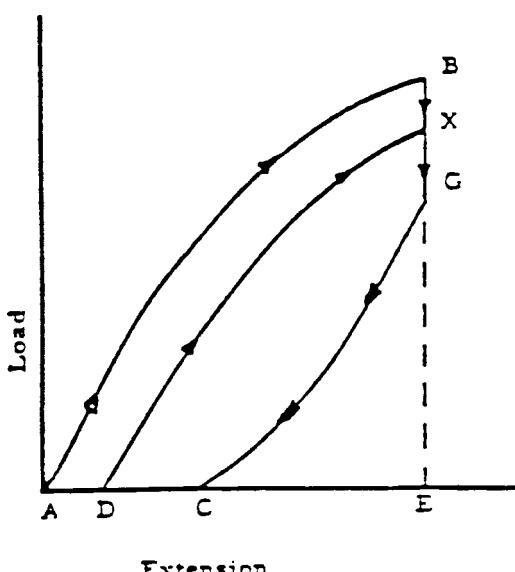
FIG. 1 Determination of the Elastic Properties of Films
