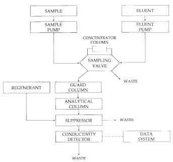
FIG. 2 Schematic of an Ion Chromatograph
