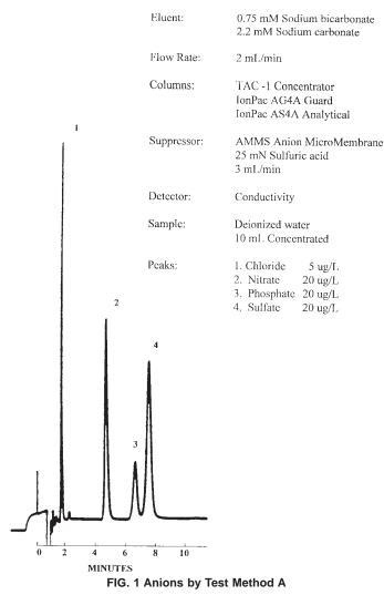
8.2 The anions are identified based on their retention times, when compared to known standards. Quantitation is accomplished by measuring the peak height or area and comparing it to a calibration curve generated from known standards.
