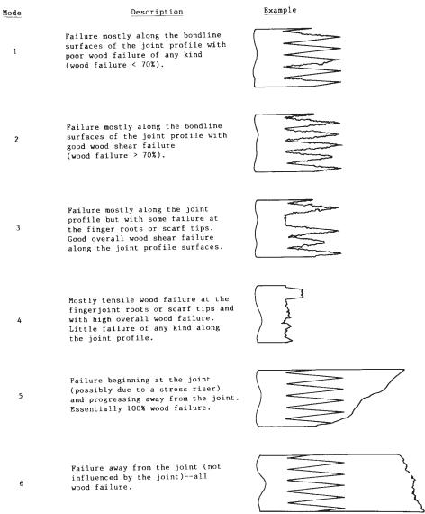
FIG. X3.1 Failure Mode Criteria
