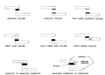
FIG. 1 Sketches Representing Failure Modes
