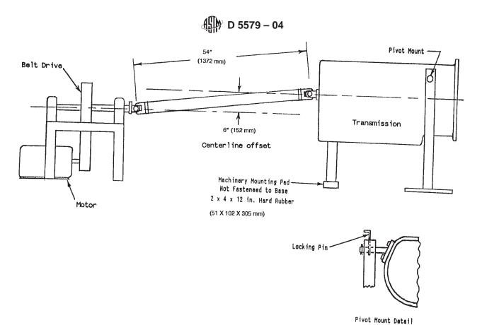
FIG. 2 Typical Layout of Drive System
