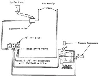
FIG. 6 Air Control and Supply System
