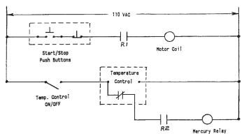
FIG. 8 Typical Schematics of Safety Circuits
