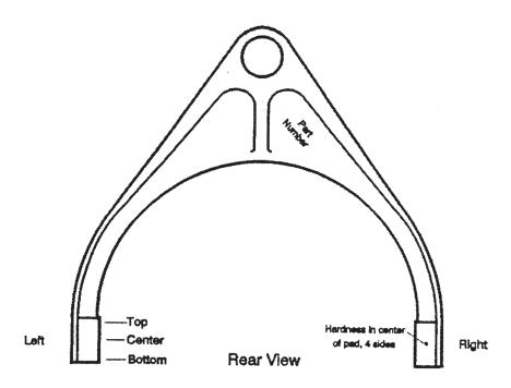
Note 1—Side of fork with forged angle and part number is the rear side. View the fork from this side to identify the pads as left and right.
