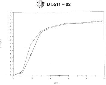
FIG. 3 Representative Plot Showing Total Biogas Production from Inoculum Plus Cellulose for Three Replicate Specimens Tested in a Single Run
