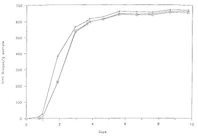
FIG. 4 Representative Plot Showing Net Biogas Production from Cellulose for Three Replicate Specimens Tested in a Single Run
