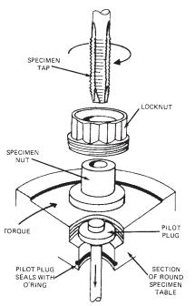
FIG. 3 Exploded View of Specimen Alignment
