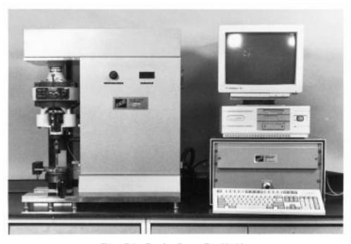
FIG. 2 Falex Tapping Torque Test Machine
