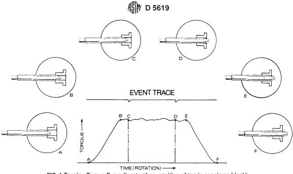
FIG. 1 Tapping Torque Curve (insets show position of tap in specimen blank)
