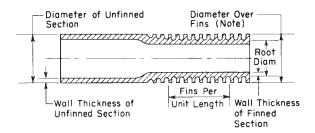
Note 1—The diameter over the fins shall not exceed the diameter of the unfinned section unless otherwise specified.
