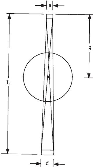
FIG. 14 A Sketch Illustrating the Geometry of the X-Ray Beam of a CT Scanner, Where  $d$  is the Detector Width,  $a$  is the X-Ray Source Width,  $L$  is the Distance Between the Source and the Detector, and  $q$  is the Distance Between the Source and the Imaging Point
