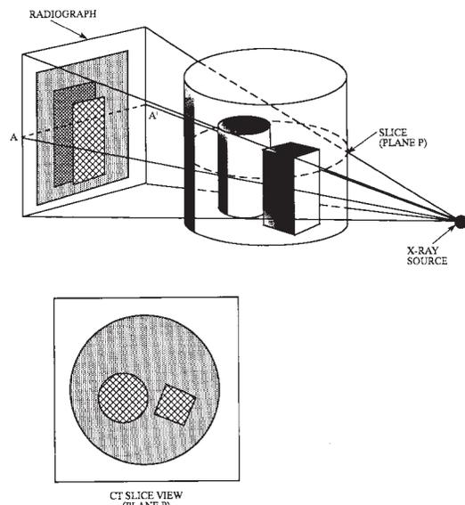
**FIG. 1 A CT Image Versus a Conventional Radiograph**
