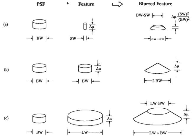
FIG. 15 A Sketch Illustrating the Two-Dimensional Convolution of a Point-Spread Function (PSF) of Diameter  $BW$  with Features of Varying Diameters: (a)  $SW < BW$ , (b)  $BW = BW$ , and (c)  $LW > BW$ . The Symbol (\*) Represents the Convolution of Two Functions
