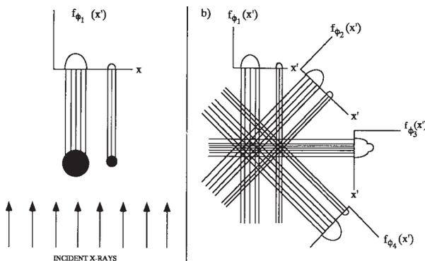
FIG. 2 Schematic Illustrations of How CT Works
