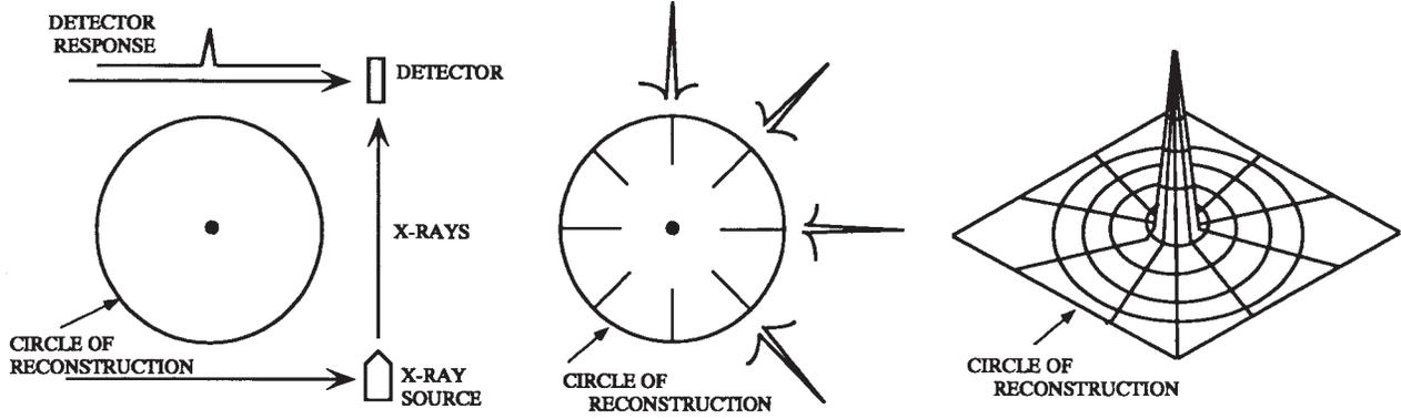
A. PROJECTION OF POINT OBJECT      B. FILTERED BACK PROJECTION TECHNIQUE      C. RECONSTRUCTION IMAGE OF A POINT
