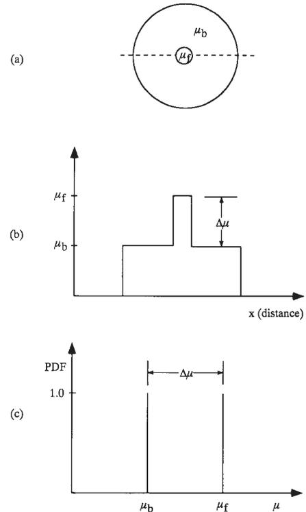
FIG. 13 (a) A Sketch Illustrating a CT Reconstruction of a Small Feature of Attenuation Coefficient  $\mu$ , Embedded in the Center of a Background Material of Attenuation Coefficient  $\mu_b$ ; (b) A Plot of the CT Density Profile Through the Feature in (a); and (c) A Probability-Distribution Function (PDF) for the Attenuation Coefficients Found in (a)
