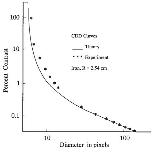
**FIG. 21 A Comparison Between Predicted and Measured CDD Curves for a Real Scanner; The Object Scanned is an Iron Cylinder of Radius 2.54 cm that is Irradiated By 0.8-MeV X-ray Photons; A Value of 8.5 was used for the Constant  $c$  in Eq 25 and its Derivative Equations**
