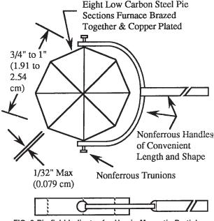
FIG. 3 Pie-field Indicator for Use in Magnetic Particle Examination
