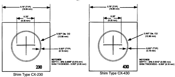
FIG. X2.1 Shims for Magnetic Particle Testing
