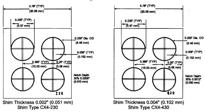
FIG. X2.3 Shims for Magnetic Particle Testing
