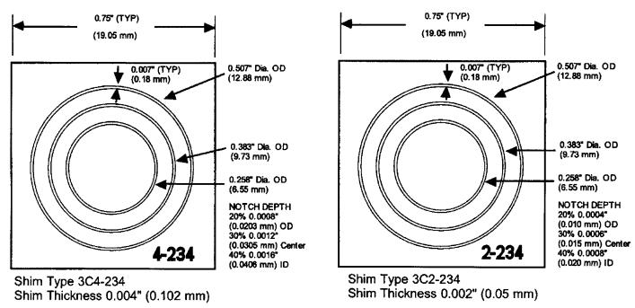
FIG. X2.2 Shims for Magnetic Particle Testing
