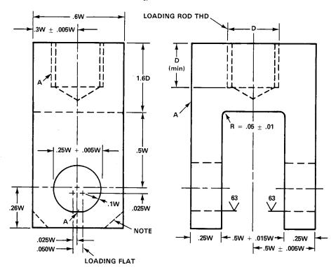
A - SURFACES MUST BE FLAT, IN-LINE & PERPENDICULAR, AS APPLICABLE TO WITHIN 0.002 IN T.I.R. (.05 mm)
