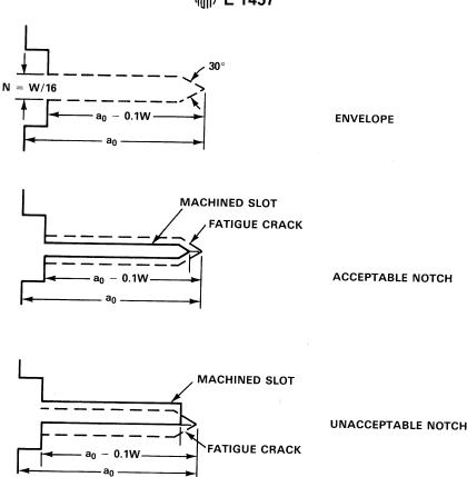
Note 1—N, need not be less than 1.6 mm (1/16 in.) but must not exceed W/16.
