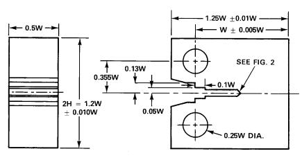
COMPACT TEST SPECIMEN FOR PIN OF 0.24W (+0.000W/-0.005W) DIAMETER FIG. 1 Drawing of a Standard C(T) Specimen
