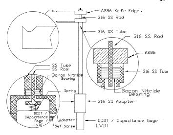
Note 1—The rod and tube must be made from the same material.
