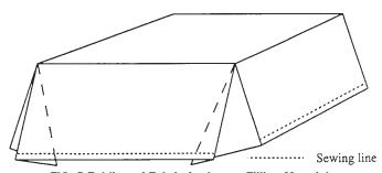
FIG. 5 Folding of Fabric for Loose Filling Materials
