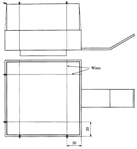
FIG. 4 Assembling of Specimen Upholstered with Leather
